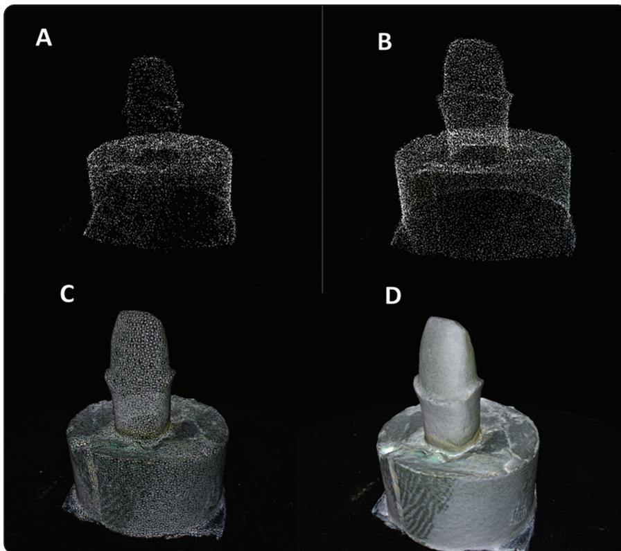
Fig. (5) Reconstruction of three-dimensional model. A: Sparse point cloud, B: Dense point cloud, C: Mesh construction & D: Textured mesh.
