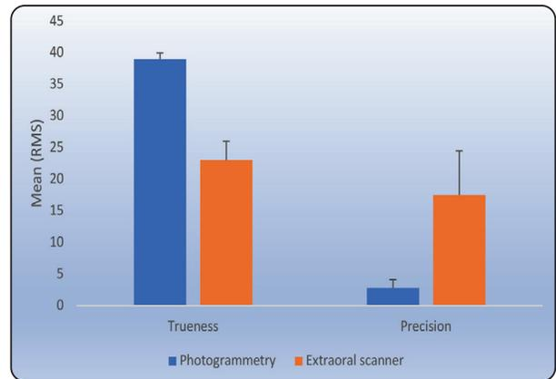
Fig. (7) Bar chart showing deviation results for trueness and precision in microns
