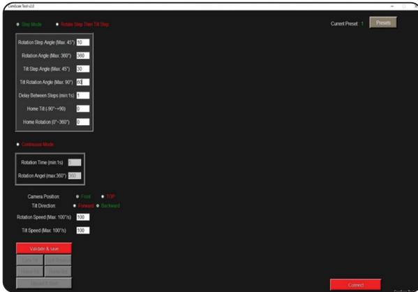
Fig. (4) Graphical user interface (GUI) used for controlling the turntable device.
