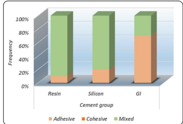
Fig.(4) Frequency distribution of failure modes analysis (%) in tension
