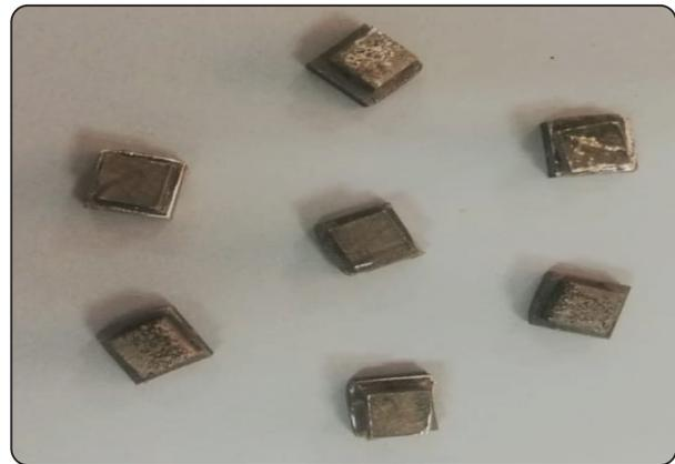
Fig. (2) Cemented CrCo-Titanium plates for shear bond strength test
