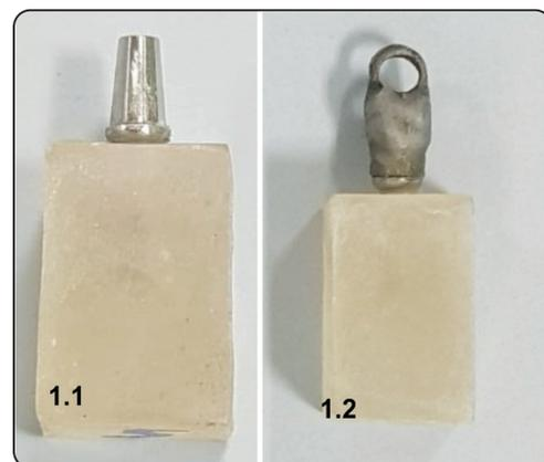
Fig. (1) (1.1) The Titanium implant analogue mounted in acrylic resin block. (1.2) The Co-Cr Coping is fitted on the implant analogue
