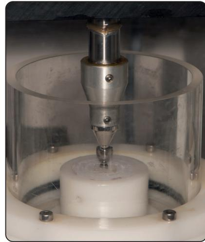
Fig. (3): Effect of chewing simulator on straight MU abutment
