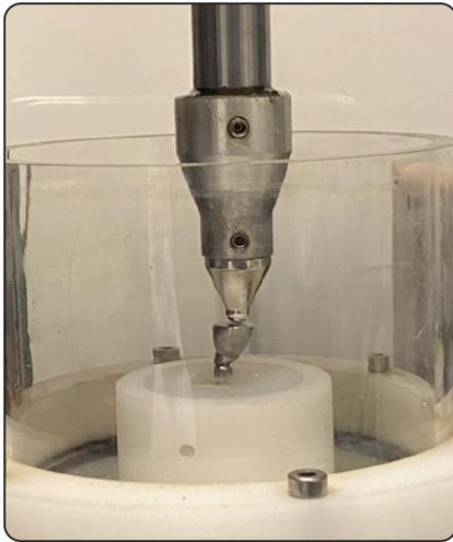
Fig. (2): Effect of chewing simulator on 17 degree angled MU abutment
