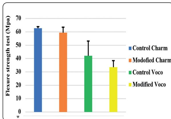
Fig. (3): Histogram showing a comparison of the flexural strength in modified and control samples.
