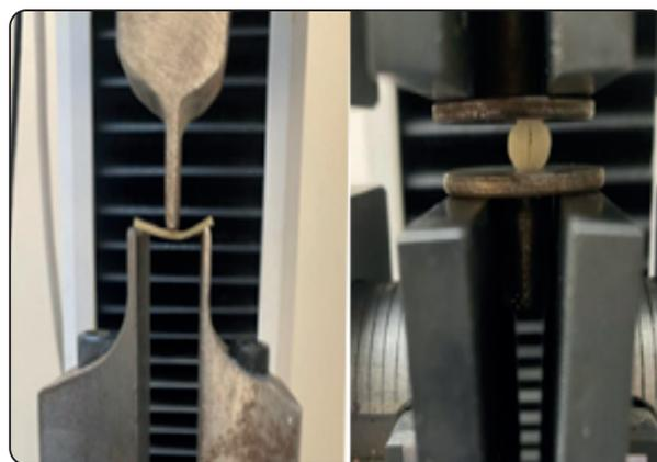
Fig. (1). Measurement of flexural strength and diametral tensile strength
