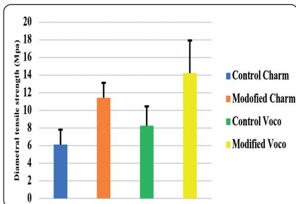
Fig. (2): Histogram showing a comparison of the diametral tensile strength in modified and control samples.
