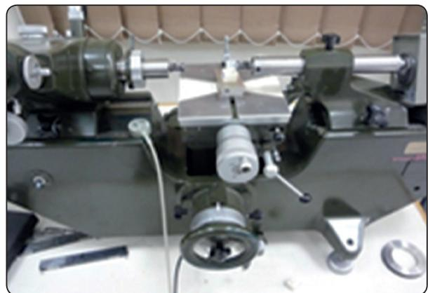
Fig (2): Universal horizontal metroscope
