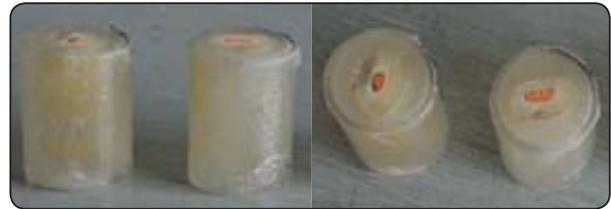
Fig. (2) Roots embedded in self cure acrylic resin, centralized in standardized tubes.
