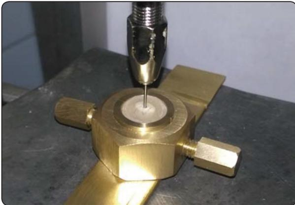
Fig. (4): Slice sample seated in the lower part of the testing machine and a cylindrical stainless steel plunger of 0.8 mm diameter in the upper part.
