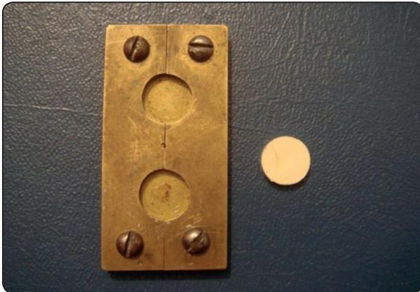
Fig. (1) Split circular brass mold used to create disc samples.
