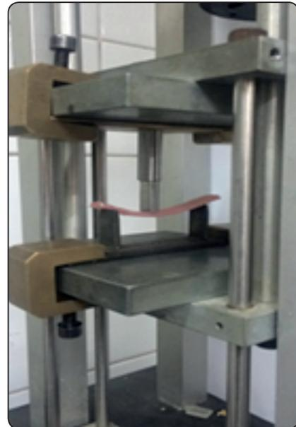
Fig. (1) Universal testing machine during testing
