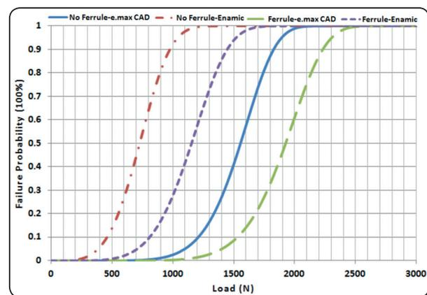
Fig. (5) A graph showing failure probability vs. load curves of the four tested groups.
