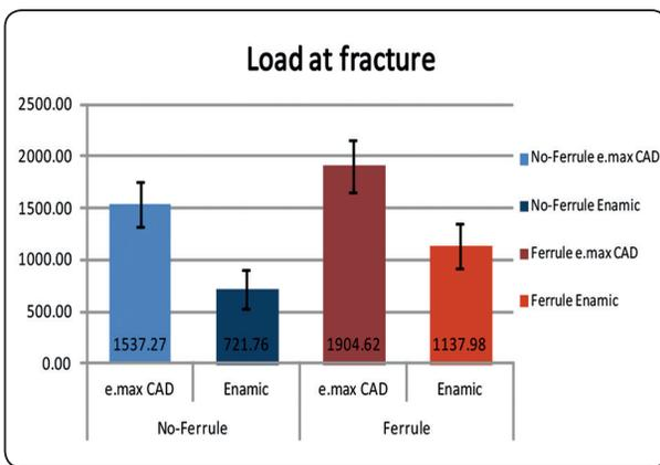
Fig. (3) Histogram of load at failure mean values (N) with standard deviation bars for the tested subgroups.
