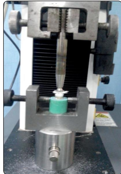
Fig. (2) A sample in the universal testing machine.
