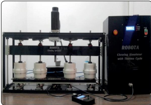
Fig. (1) The chewing simulator with chambers containing some samples.
