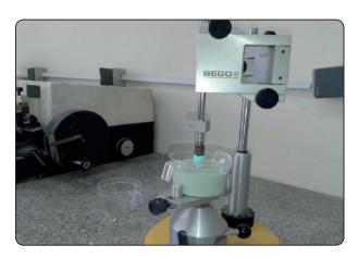
Fig. (1): Milling surveyor used to mount the tooth in the mold
