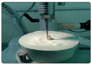
Fig. (2) Milling surveyor used in tooth preparation
