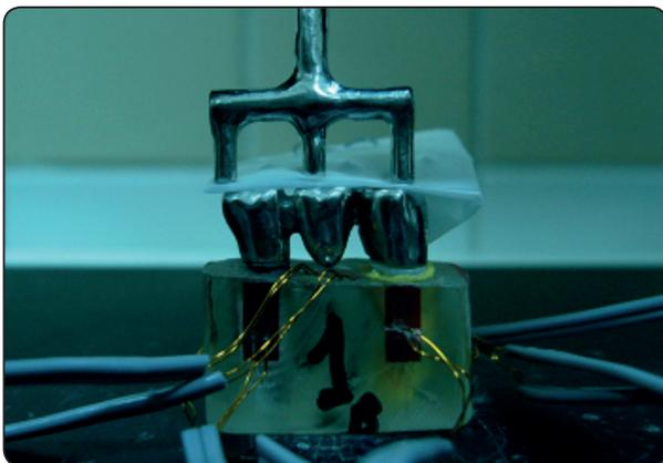
Fig. (2) Model assembly on platform of universal testing machine with fork attachment
