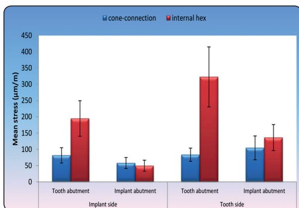
Fig. 3. Bar chart representing mean and standard deviation values of strains induced using the two implant systems
