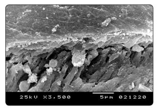
Fig. (3) SEM image, 3500x, showing precipitation of nano hydroxy apatite particles on spattered enamel surface and covered by bonding agent. This group suffered from micro-gap formation at tooth adhesive interface.
