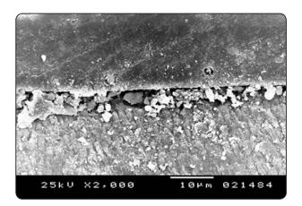
Fig. (4) SEM image, 2000x, showing micro-gap formation at tooth adhesive interface after spattering of nanoparticles.
