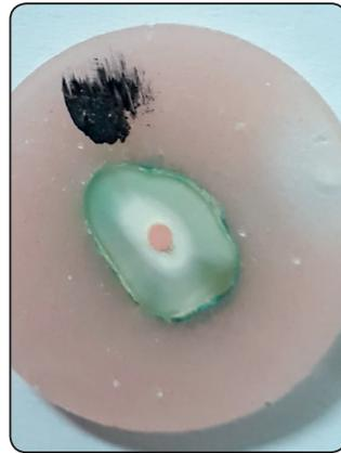
Fig. (2): Root sample after insertion in acrylic blocks
