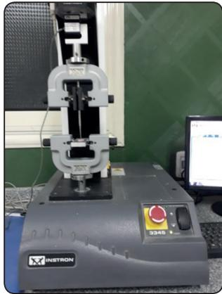
Fig. (1): Instron machine used in push out test
