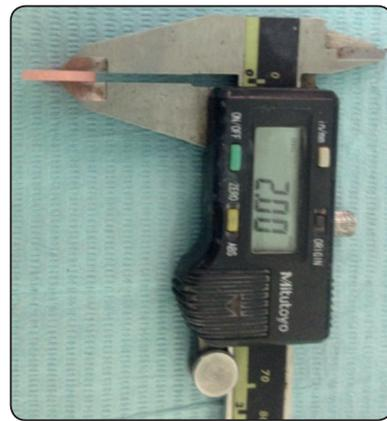
Fig. (4): Caliber checking 2 mm thickness of slices samples
