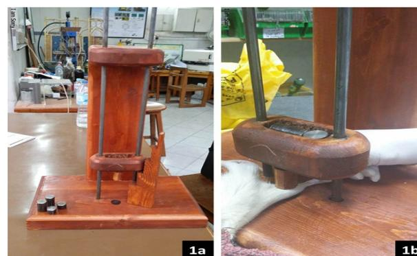
**Fig. 1a:** A photo illustrating muscle contusion device.
