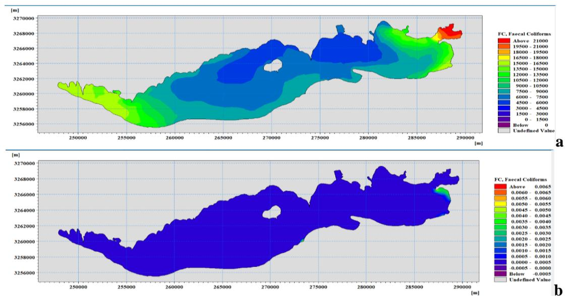
**Fig. 24.** FC simulation in spring 2021: **a)** Before treatment; **b)** After treatment
