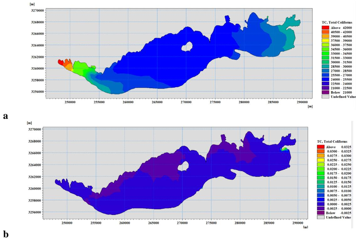
**Fig. 23.** TC simulation in spring 2021: **a)** Before treatment; **b)** After treatment
