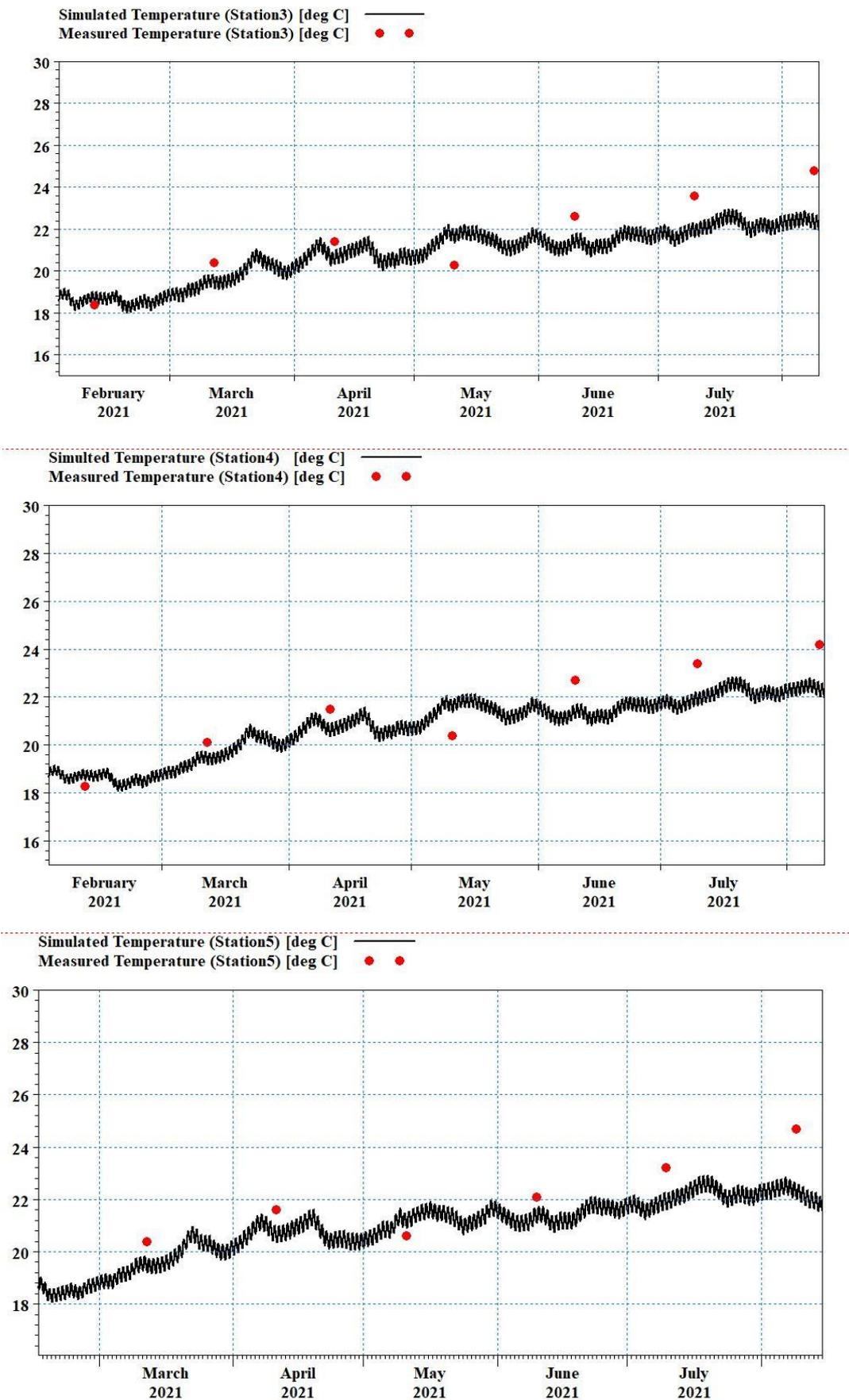
Fig. 17. Simulated and measured water temperature at the five verification sites
