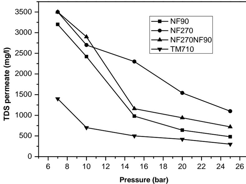
Fig. 7. Variation in TDS permeate concentration with applied pressure
