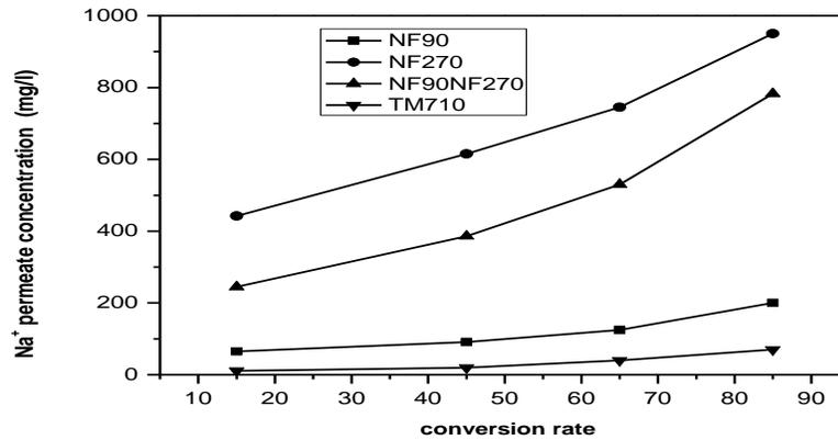
**Fig. 11.** Variation of  $\text{Na}^+$  concentration in permeate with conversion rate
