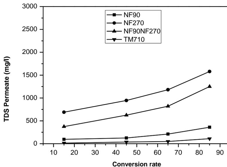
**Fig. 9.** Variation in permeate TDS as a function conversion rate
