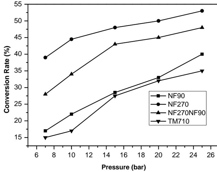
**Fig. 3.** Variation of conversion rate (Y%) as a function of applied pressure
