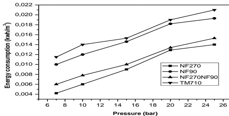
Fig. 8. Variation in energy consumption with applied pressure
