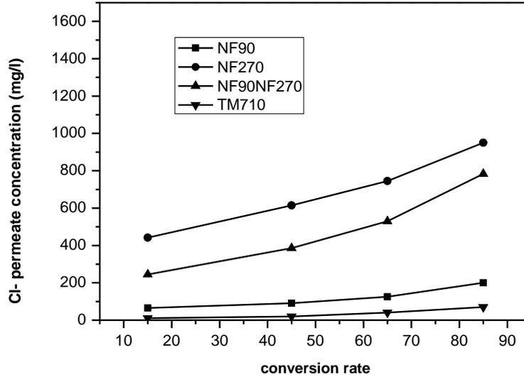
**Fig. 10.** Variation of  $\text{Cl}^-$  concentration in permeate with conversion rate
