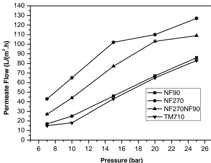
**Fig. 2.** Variation of permeate flow as a function of applied pressure
