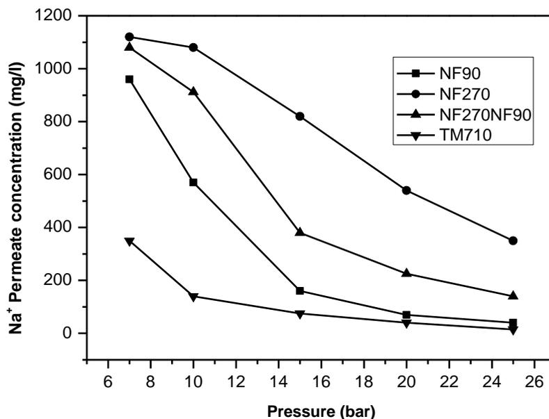
Fig. 5. Variation of Na<sup>+</sup> permeate concentration as a function applied pressure
