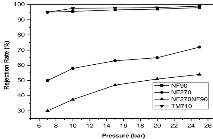
**Fig. 4.** Variation of the overall rejection rate as a function of applied pressure
