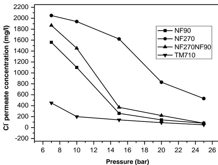
Fig. 6. Variation of Cl<sup>-</sup> permeate concentration with applied pressure
