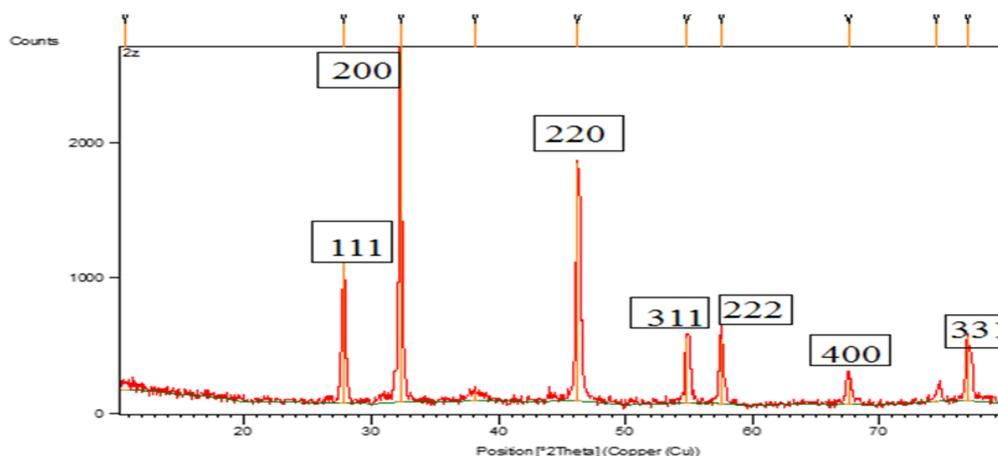
**Fig. 13.** X-ray diffraction of the nanoparticles fabricated from the extract of *E. intestinalis*
