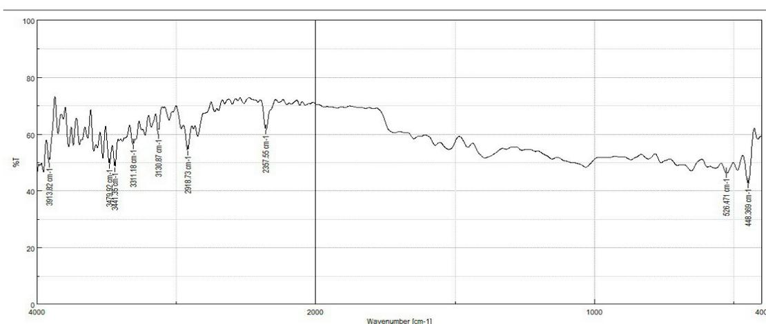
**Fig. 10.** Infrared spectrum of the nanoparticles fabricated from the extract *E. intestinalis*
