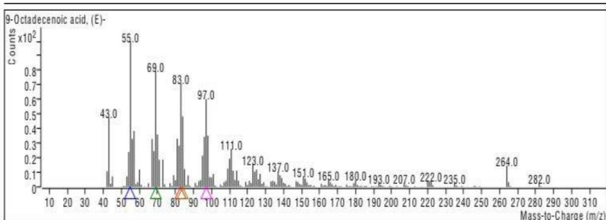
**Fig. 6.** Mass spectrum of the compound oleic acid isolated from *E.intestinalis*
