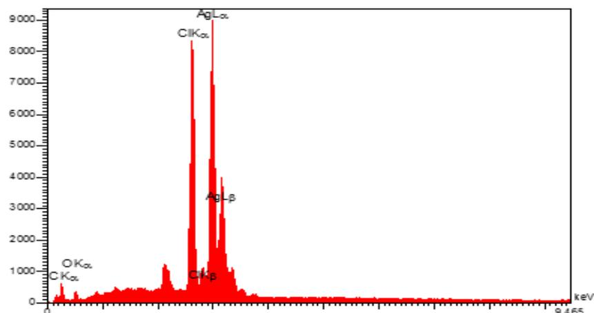
**Fig. 11.** Energy-dispersive X-ray spectroscopy analysis of the synthesized silver nanoparticles from the extract *E. intestinalis*
