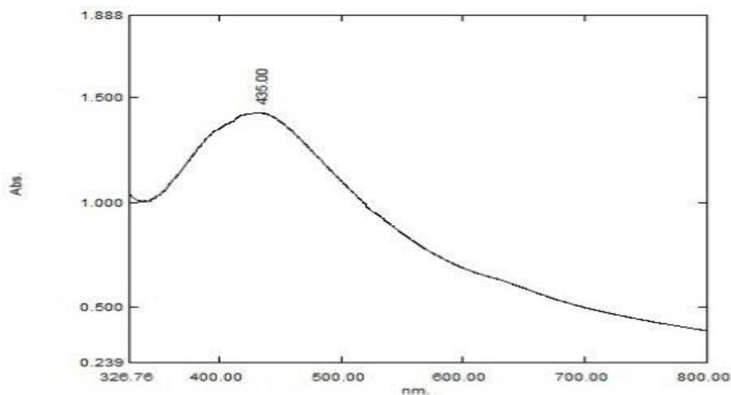
**Fig. 8.** Visible and ultraviolet absorption spectrum of *E. intestinalis*
