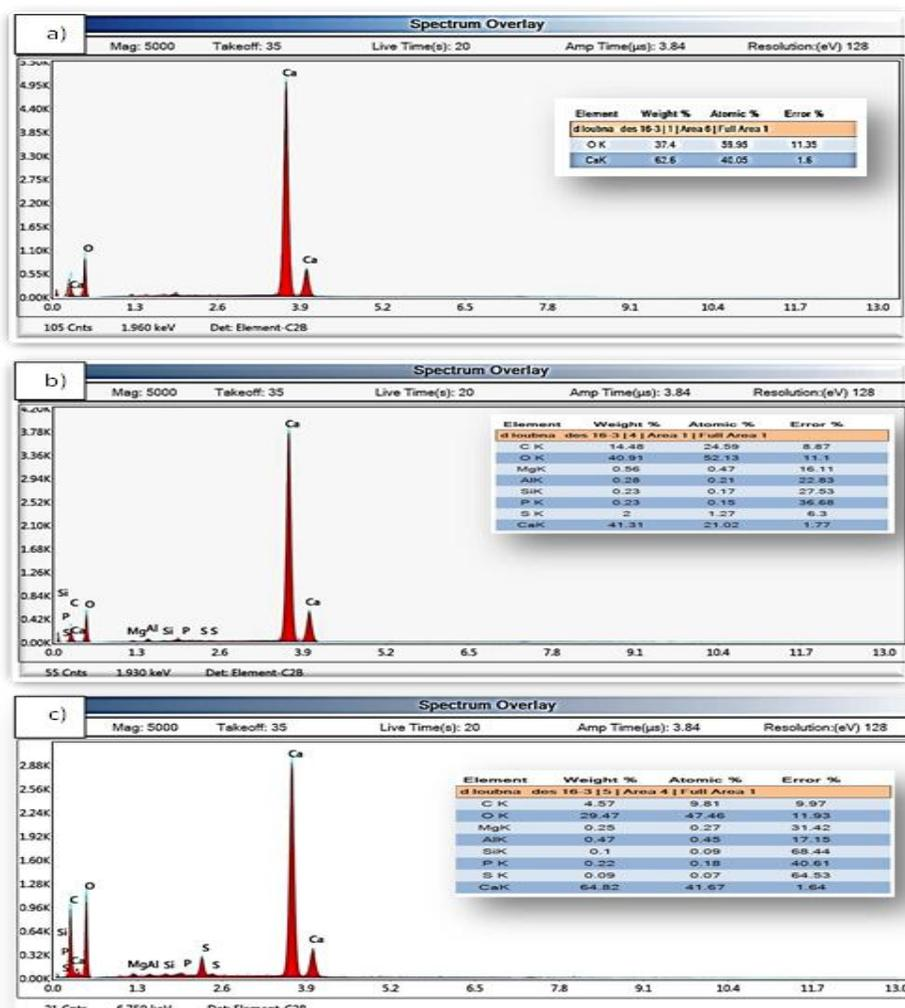
**Fig. 4.** Energy Dispersive X-Ray Analysis (EDX) of elements on the surface of Egg Shell (ESP). a) Control sample b) raw wastewater sample c) treated wastewater sample
