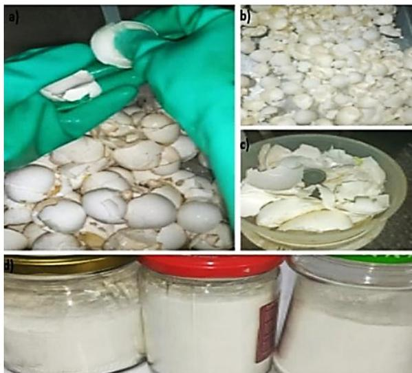
**Fig. 1.** ESP preparation steps. a) Washing eggshell, b) Drying process for eggshell at 70°C for 10 min, c) Grinding dried eggshell with an electric grinder, and d) ESP preparation
