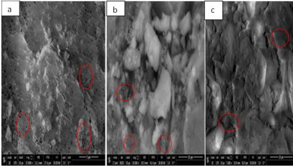
**Fig. 3.** Scanning electron microscope (SEM) investigation of ESP before and after wastewater treatment: (a) SEM for Eggshell waste powder (ESWP) as a control, (b) SEM for WESP1 (raw wastewater with ESP), (c) SEM for WESP2 (Pre-treated wastewater with ESP)
