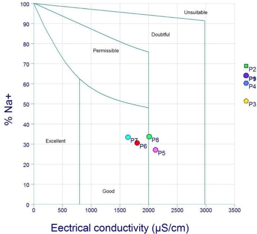
Fig. 3. Classification of groundwater according to the Wilcox diagram
