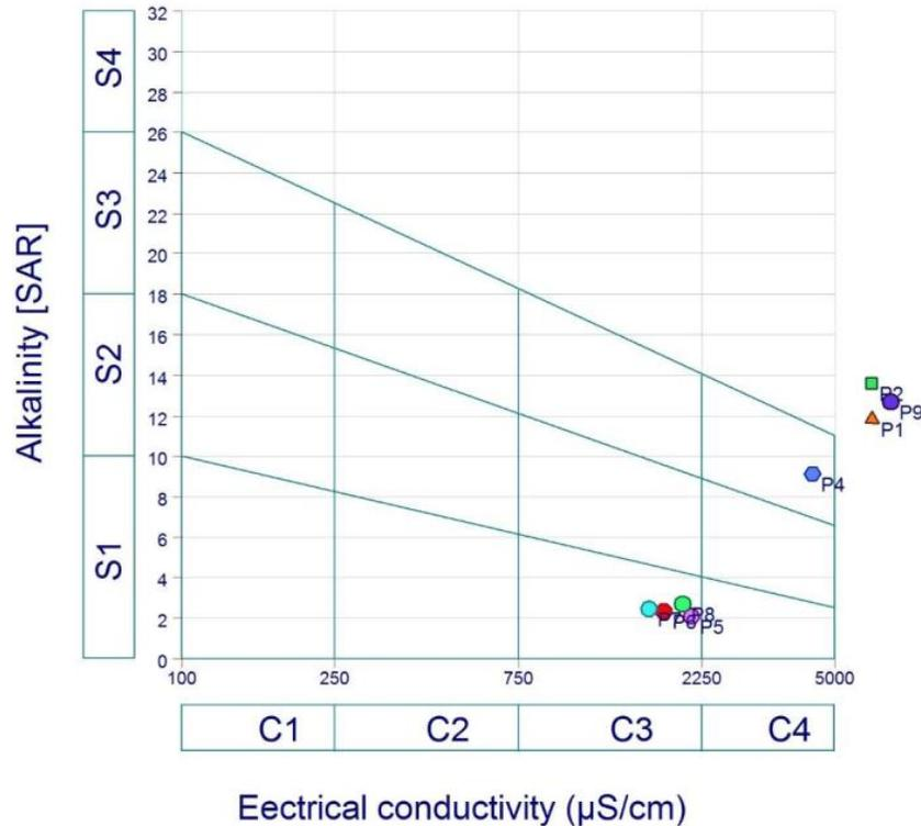
**Fig. 4.** Classification of groundwater according to the Wilcox log diagram
