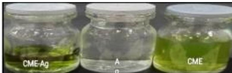
**Fig. 2.** The change in color using the *Cosmarium* methanolic extract. Ag: silver nitrate solution, CME: *Cosmarium* methanolic extract, CME-Ag (AgNPs): silver nanoparticles synthesized by *Cosmarium* methanolic extract.
