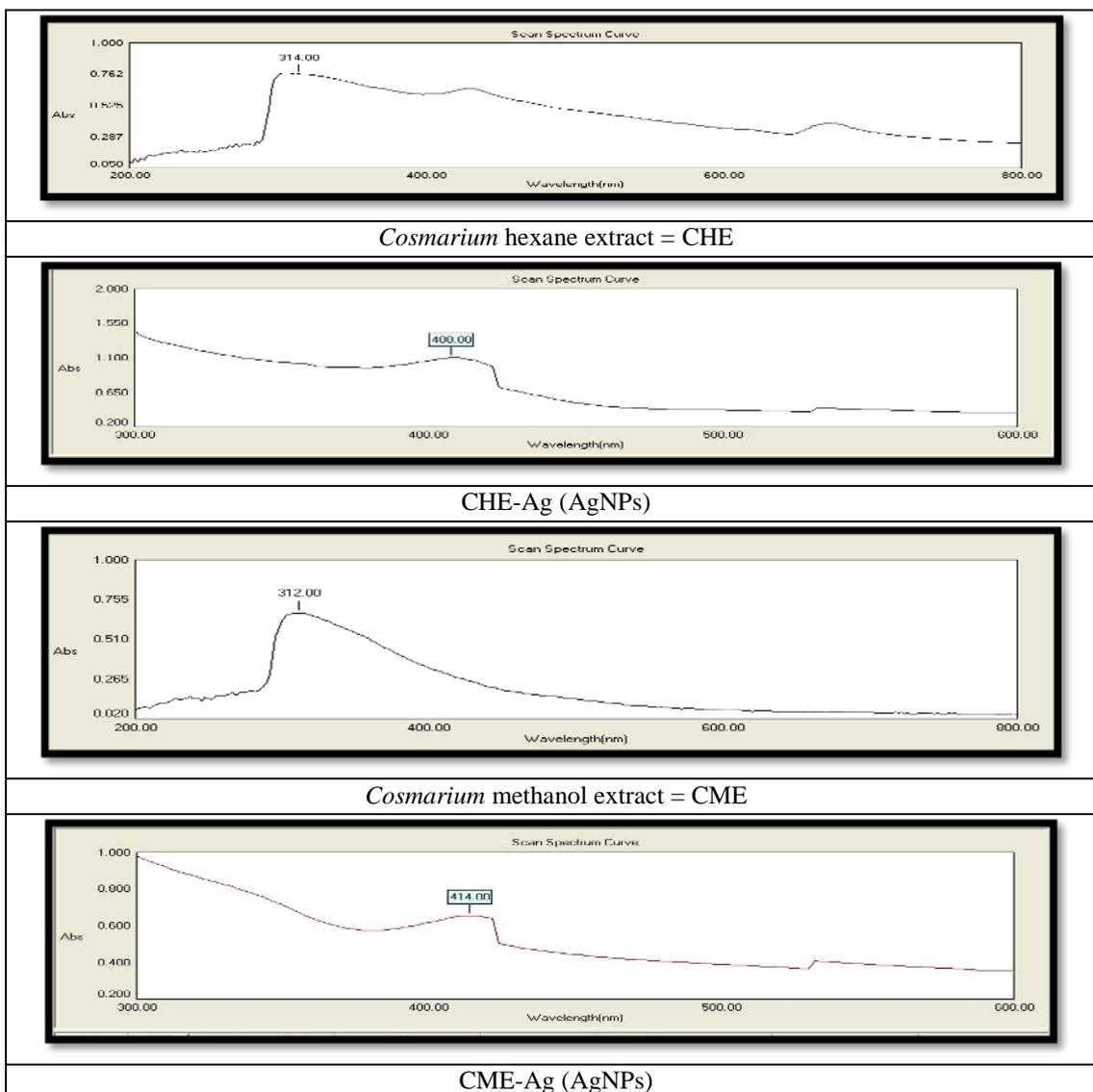
**Fig. 3.** UV-Vis spectra of AgNPs synthesized by the *Cosmarium* methanolic and hexane extracts
