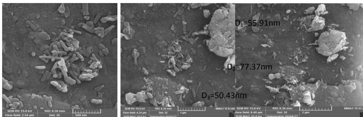
**Fig. 5.** Shape and size of silver nanoparticles (AgNPs ) synthesized by the *Cosmarium* methanolic and hexane extracts
