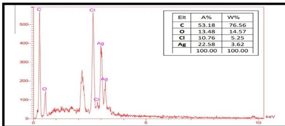
**Fig. 4.** Energy dispersive X-ray diffraction (EDX) pattern of *Cosmarium* -mediated synthesized AgNPs
