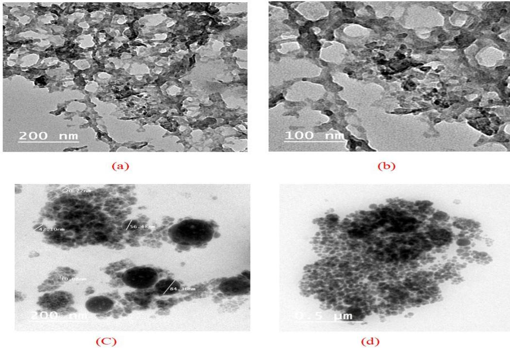
**Fig. 1.** TEM image (a,b) showing ZnO nanoparticles (ZnONPs) with size ranging from 5-15nm in diameter, and TEM image (c,d) showing selenium nanoparticles (SeNPs) of size ranging from 20- 40nm in diameter.
