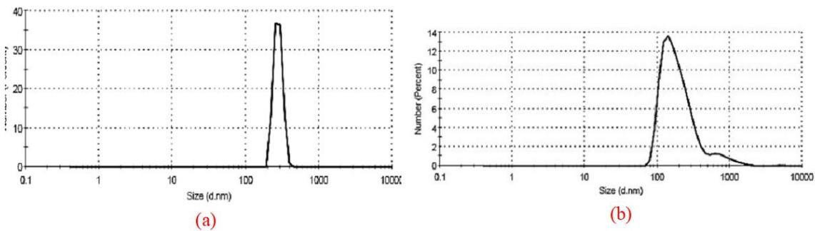
**Fig. 2.** Dynamic light scattering (a) Droplet size distribution of the ZnONPs, and (b) Droplet size distribution of the SeNPs.
