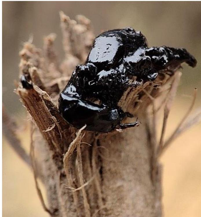
Fig. 3. Bio-oil obtained from slow pyrolysis.
