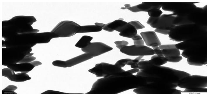
**Fig. 12. Transmission electron micrographs of synthesized ZnONPs synthesized by *E. nigrum*.**
