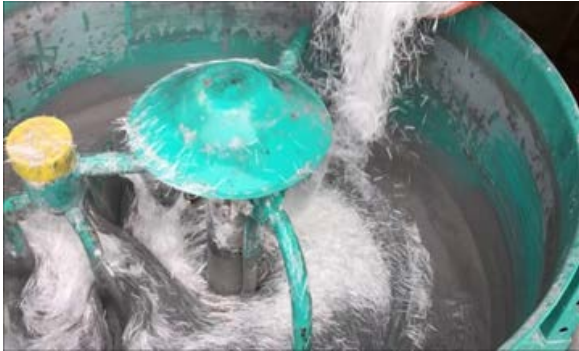
Fig. 6 Pre-chopped glass fibers mixed with concrete
