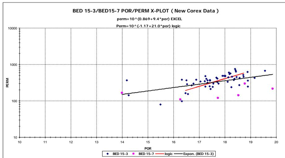
Figure 9: Cross-plot porosity-permeability with Corex data (BED-15)
