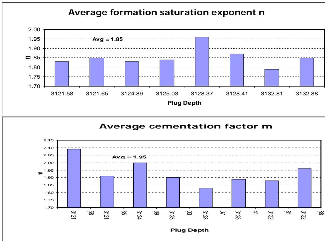
Figure 6: Formation saturation exponent n and cementation factor m.
