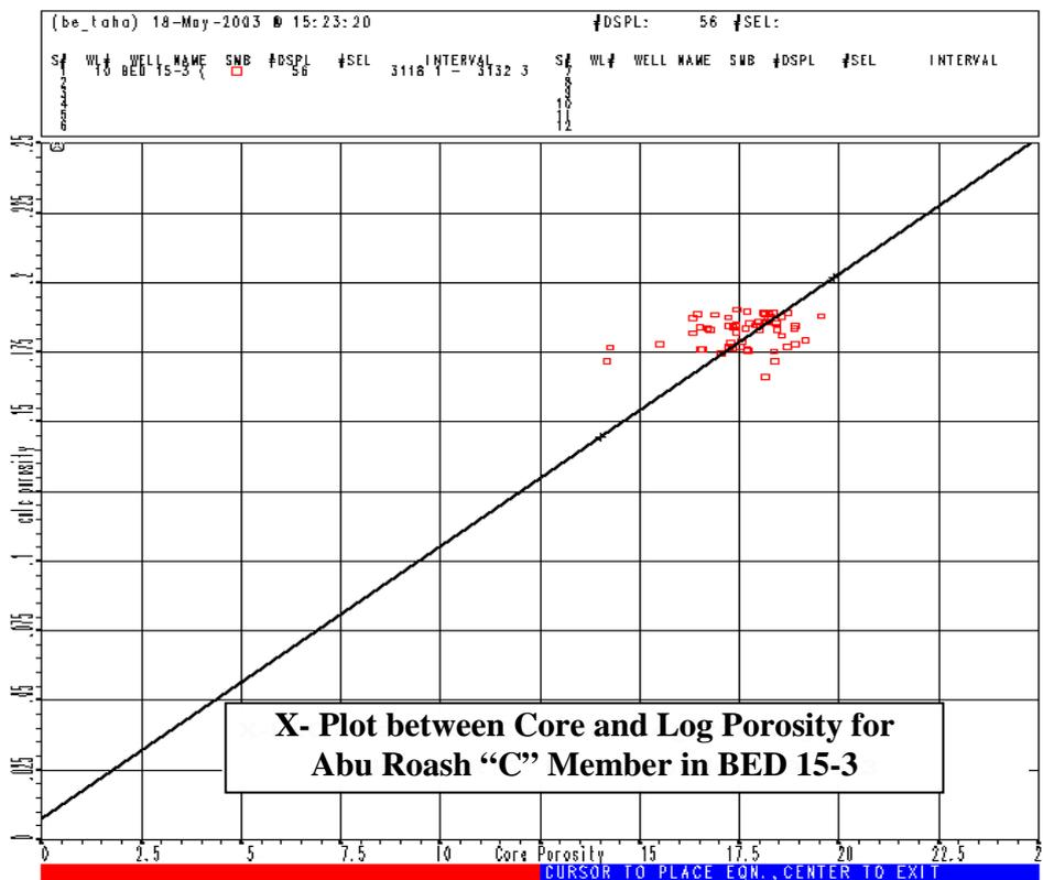
Figure 7: Cross-plot of core and log porosities (BED15-3).
