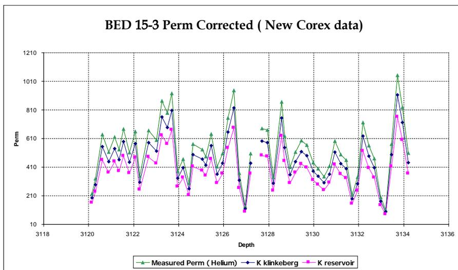
**Figure 8: Permeability corrections with Corex data (BED 15-3).**
