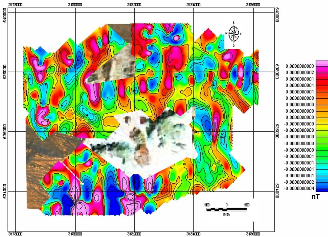
Fig. (13): Low pass frequency magnetic anomaly map.
