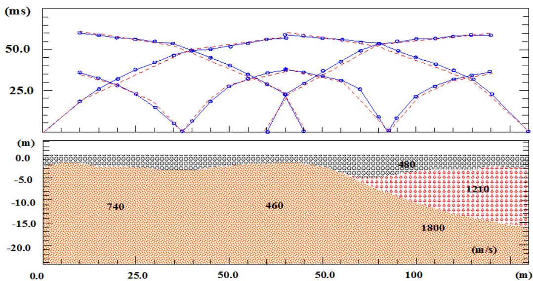
Fig. (25): 2D-seismic refraction cross-section across site NO.3.
