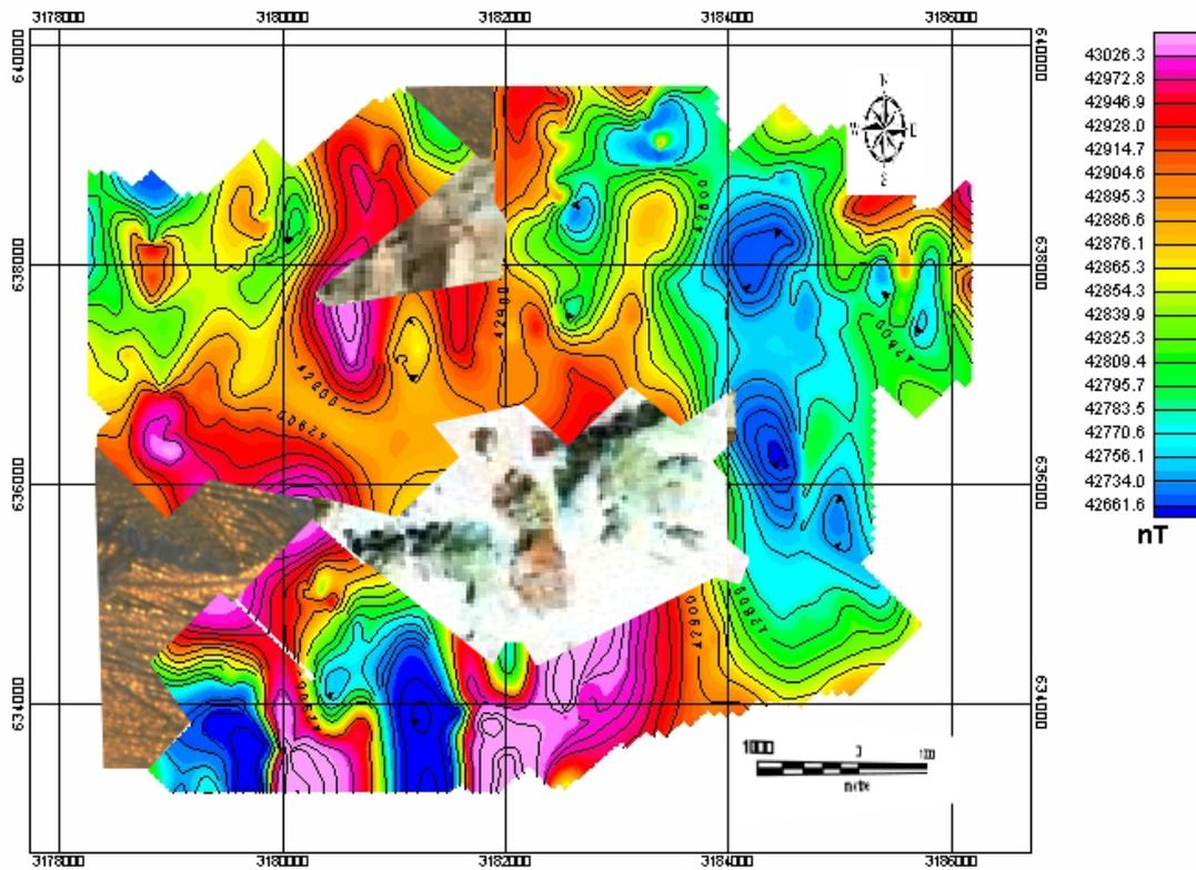
Fig. (12): Reduced to pole magnetic intensity map (R.T.P.).
