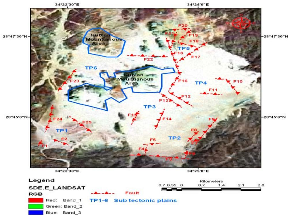
Fig. (15): Structural tectonic trends interpreted from filtering of the magnetic data.
