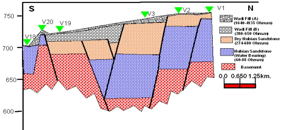
Fig. (19): Geoelectrical cross-section NO.3.
