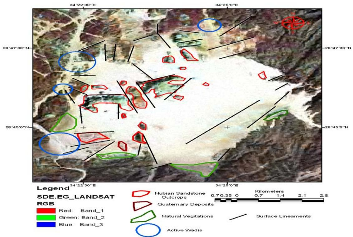
Fig. (8): Landsat image showing the interpreted groundwater indicators.
