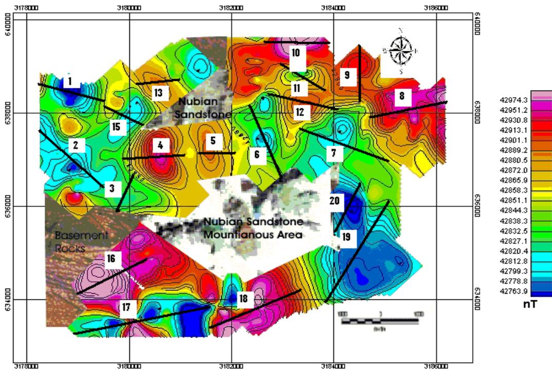
Fig. (11): Total magnetic intensity map showing locations of the spectral analysis profiles.
