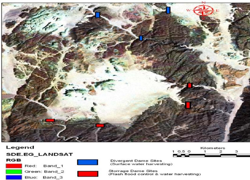
Fig. (9): Recommended dam sites for flash flood control and surface water harvesting
