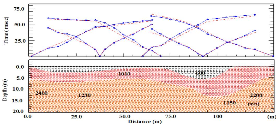
Fig. (24): 2D-seismic refraction cross-section across site NO2
