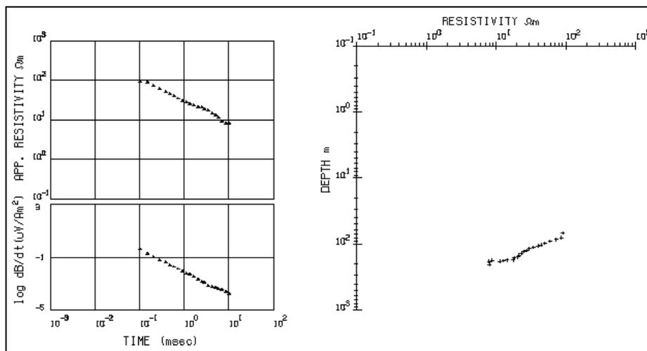
Fig 3: An example of TEM resistivity-depth transformation at sit W23.
