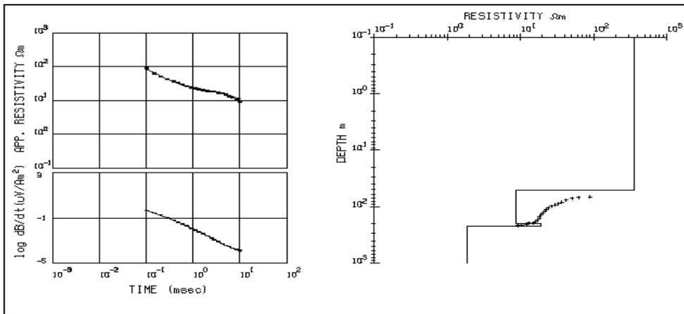
Fig.6:1-D forward and inverse modeling results of TEM data at site W8.
