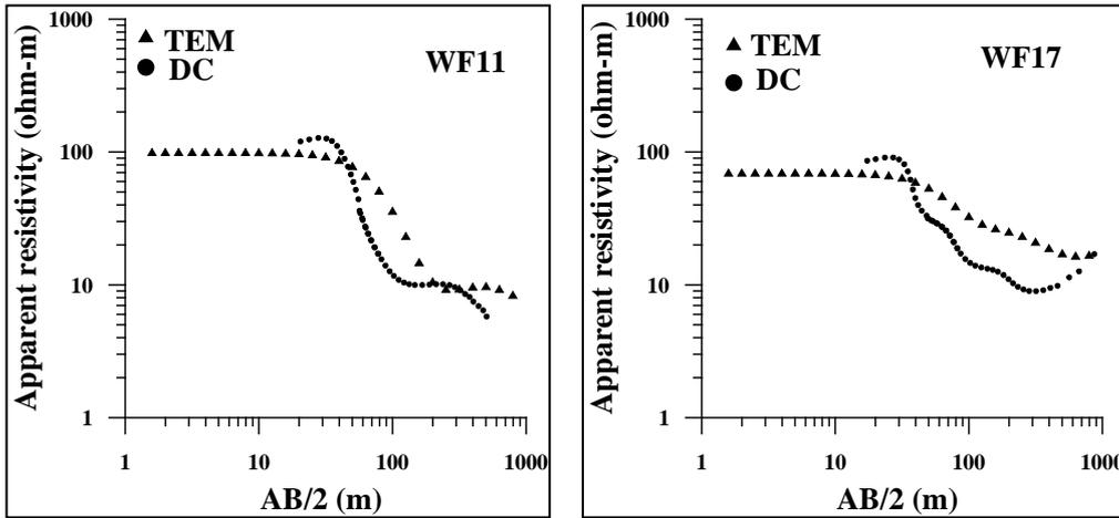
**Fig. 4: Synthetic response of broadband TEM and VES 1D apparent resistivities calculated for two borehole sites (WF11 and WF17) using the average values of the resistivities recorded in the boreholes.**
