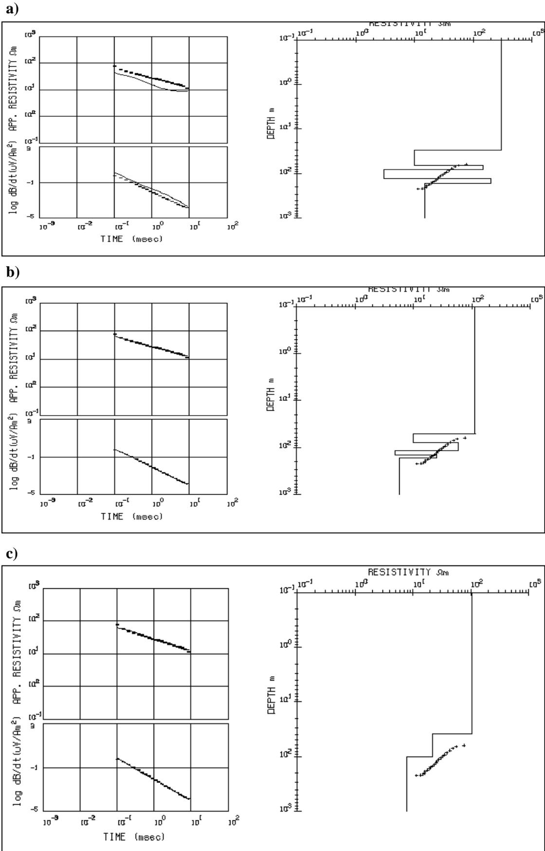
Fig. 11: Forward and inverse modeling results at site w11 beside the borehole site wf17.
