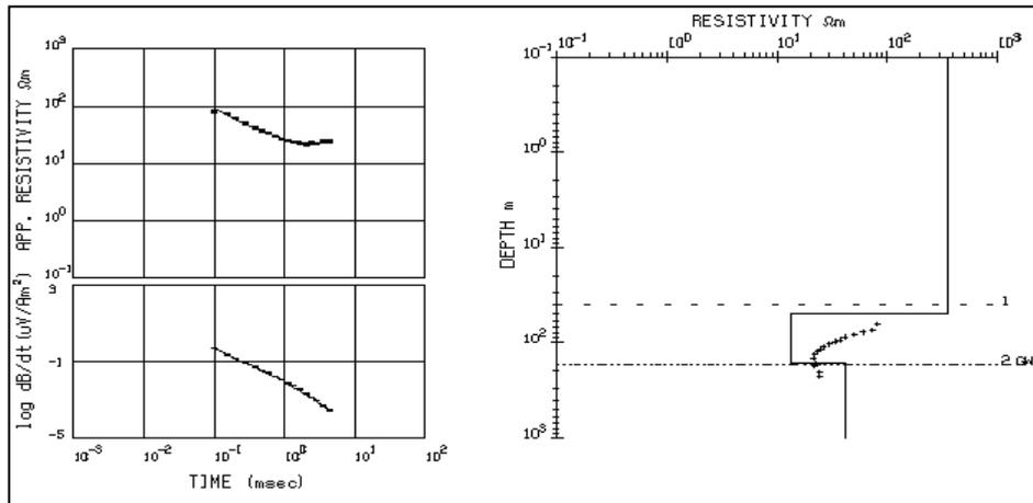
Fig. 9: 1-D inverse modeling of TEM data at site W13 beside the borehole WF11.
