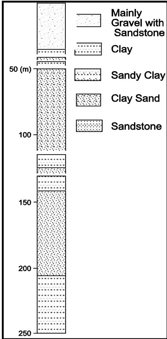
Fig. 2: Lithostratigraphic column borehole site Wf16.
