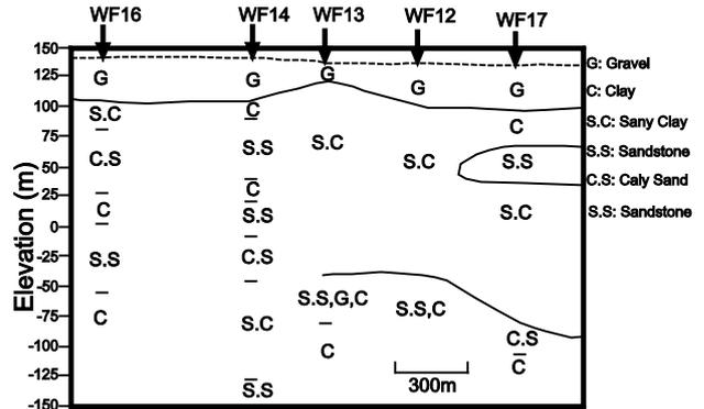
**Fig.13: Litho-stratigraphic succession at the borehole sites passing through profile A-A'**
