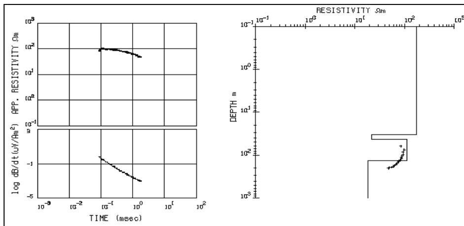
Fig. 10: 1-D inverse modeling of TEM data at site W2 150m away from borehole wF16.
