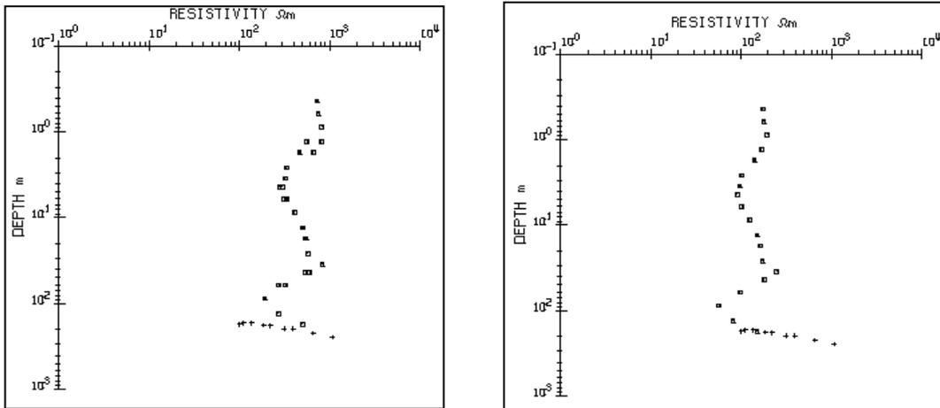
**Fig.5: DC resistivity data before and after the removal of static shift at sit wf16.**
