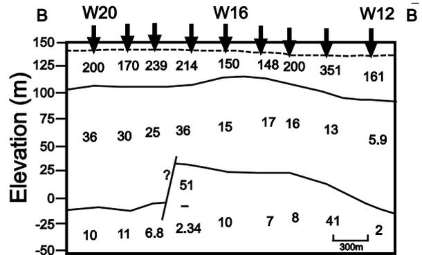
**Fig.14: 2-D geoelectric section along profile B-B' using 1-D inversion results**
