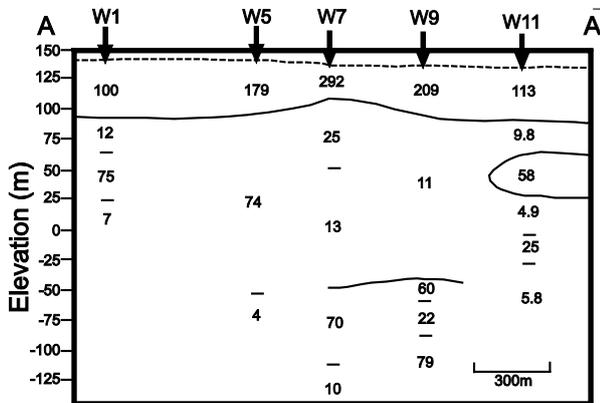
**Fig.12: 2-D geoelectric section along profile A-A' using 1-D inversion results**
