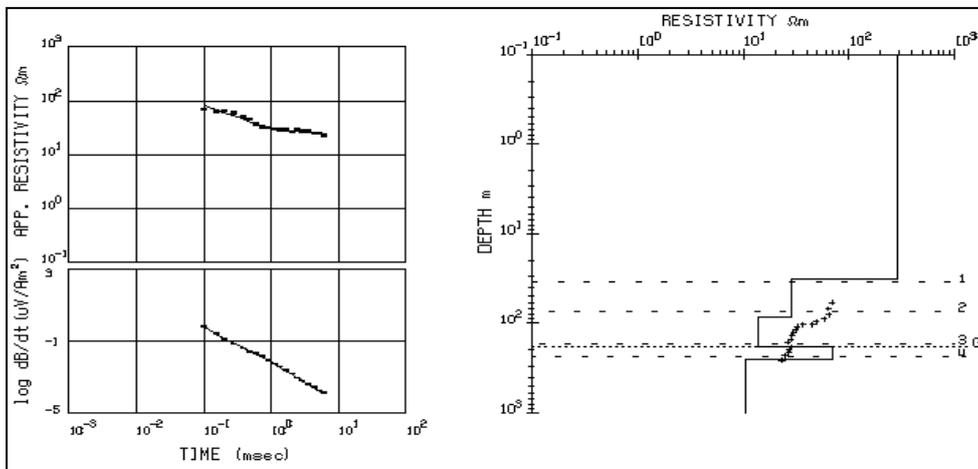
Fig. 7: 1-D inverse modeling of TEM data at site W7 beside the borehole WF13 (the lithological boundaries and depth to water are indicated).
