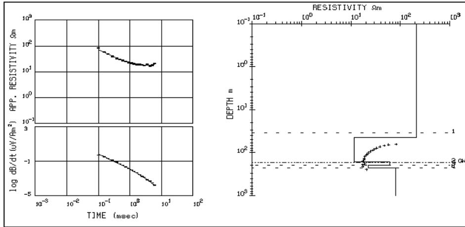
Fig.8: 1-D inverse modeling of TEM data at site W9 beside the borehole WF12.
