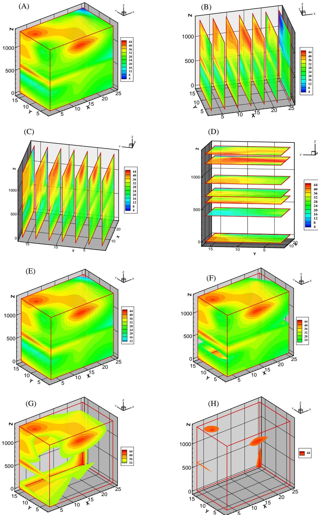
**Fig (8) Reservoir 3D Slicing and Cut Off of Movable Hydrocarbon Saturation of Abu Roash Formation in Tiba Area, Western Desert, Egypt.**
