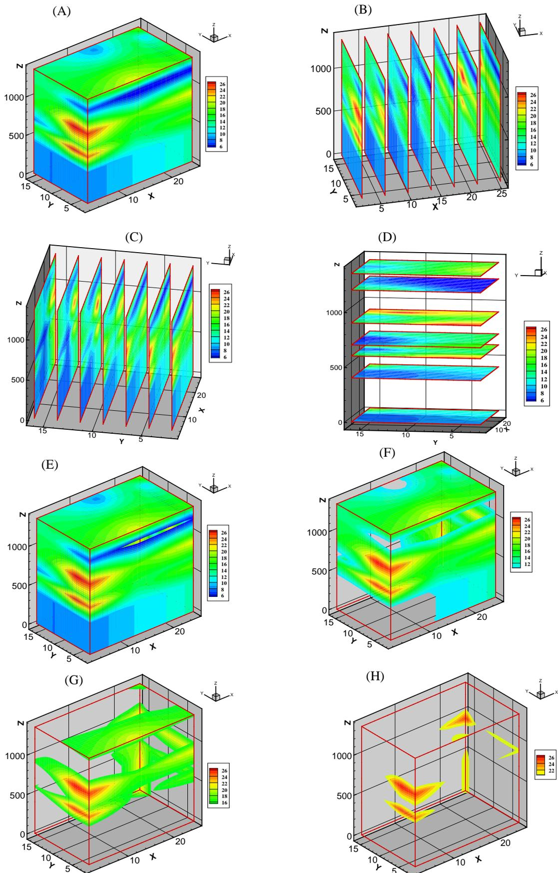
Fig (4) Reservoir 3D Slicing and Cut Off of Effective Porosity of Abu Roash Formation in Tiba Area, Western Desert, Egypt.
