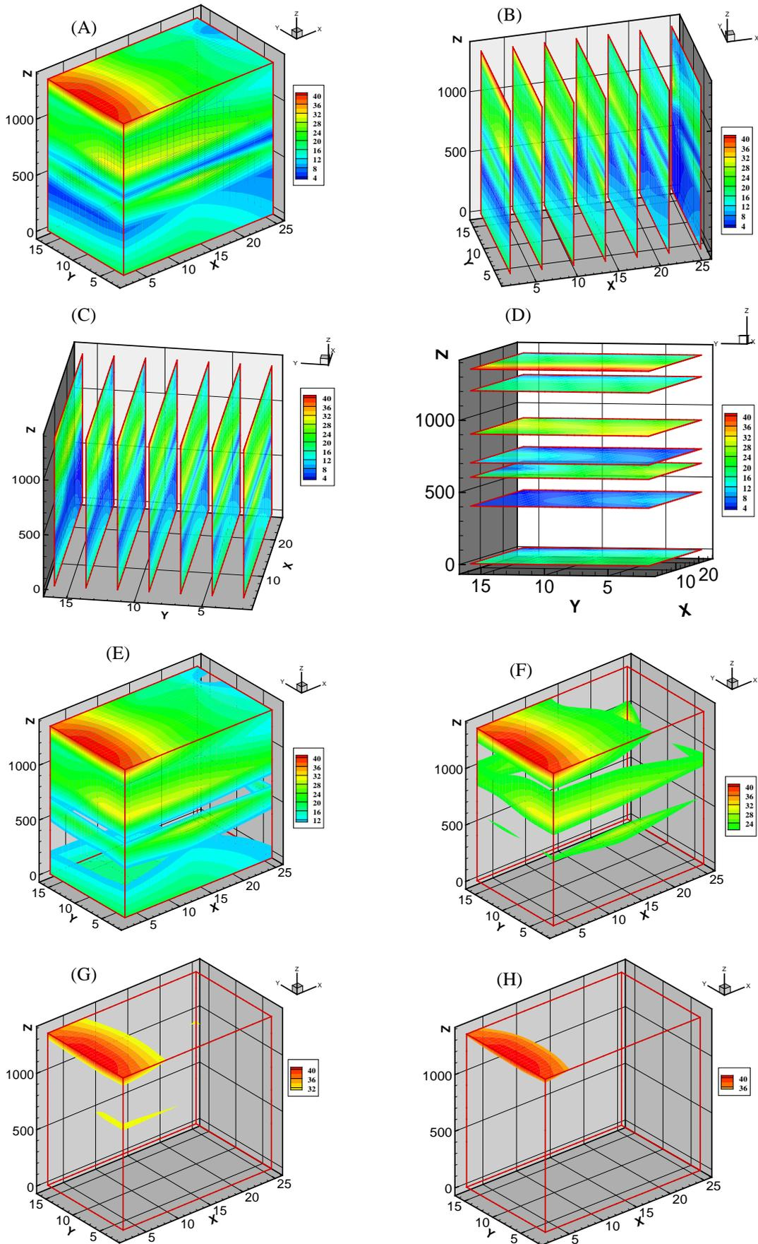
**Fig (3) Reservoir 3D Slicing and Cut Off of Shale Volume (Vsh) of Abu Roash Formation in Tiba Area, Western Desert, Egypt.**
