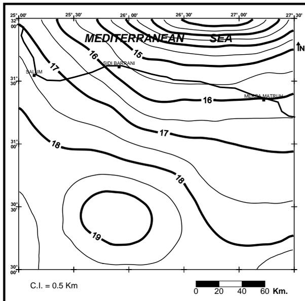
Fig. (18) Conrad depth map of the study area as interpreted from the modeled profiles.
