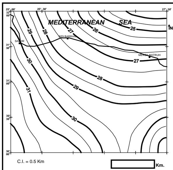
Fig. (19) Moho depth map of the study area as interpreted from the modeled profiles.
