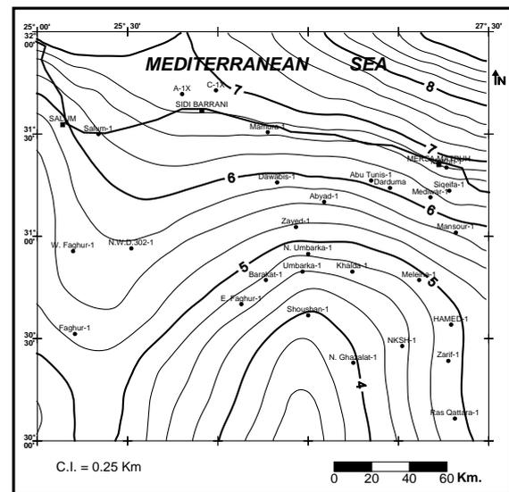
Fig. (17): Regional basement depth map of the study area as interpreted from the modeled profiles
