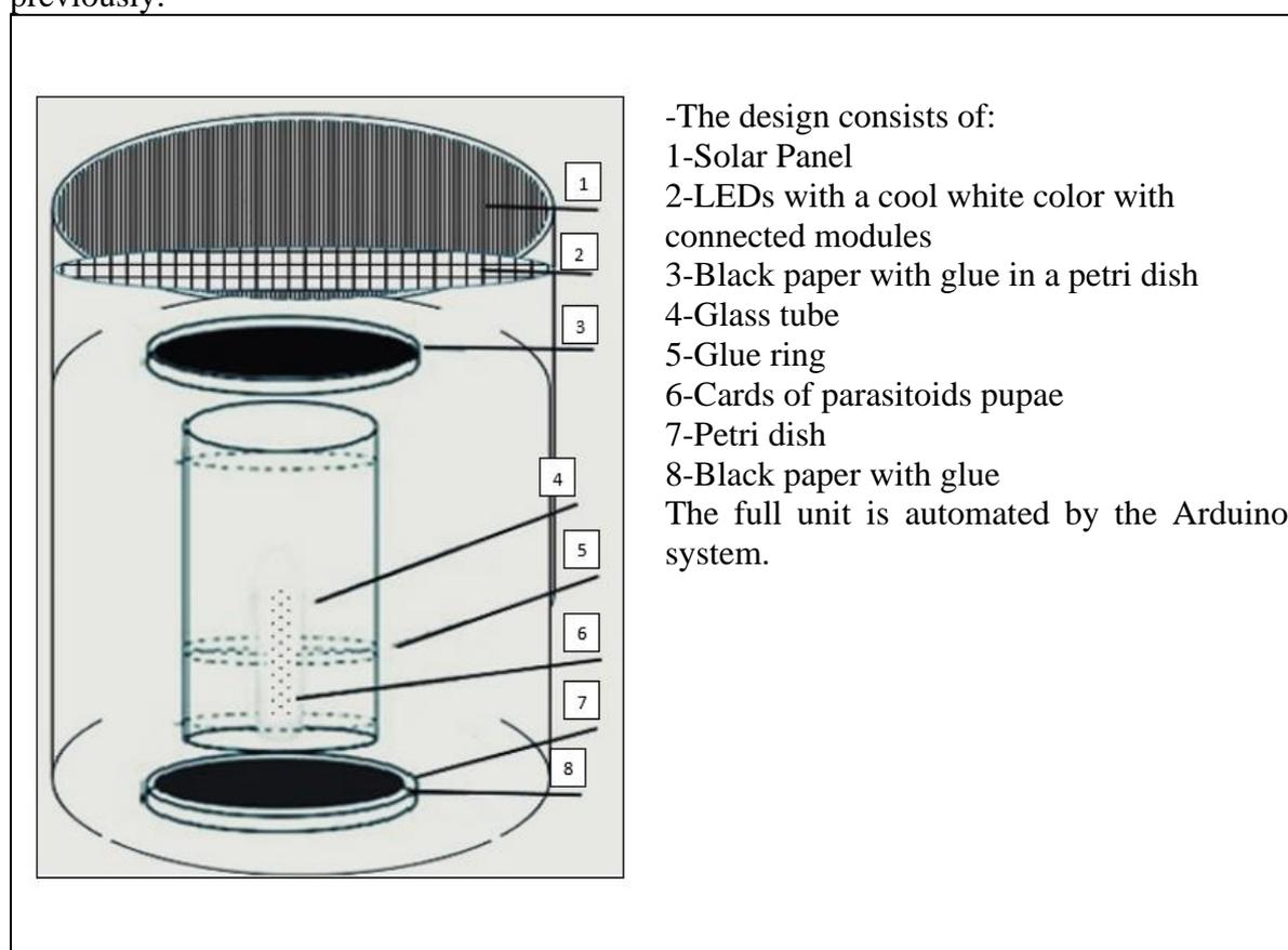
Fig.3: Automated ESALQ model unit to test the flight capacity of egg parasitoids.
