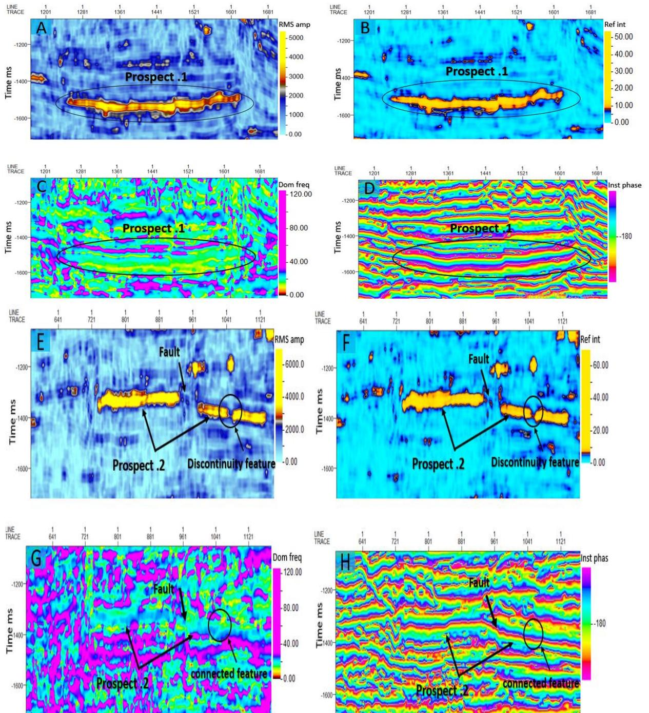
**Fig. 5: Results of the A: Root mean square amplitude, B: Reflectivity intensity, C: Instantaneous frequency, D: Instantaneous phase, applied on prospect.1 where E: Root mean square amplitude, F: Reflectivity intensity, G: Instantaneous**
