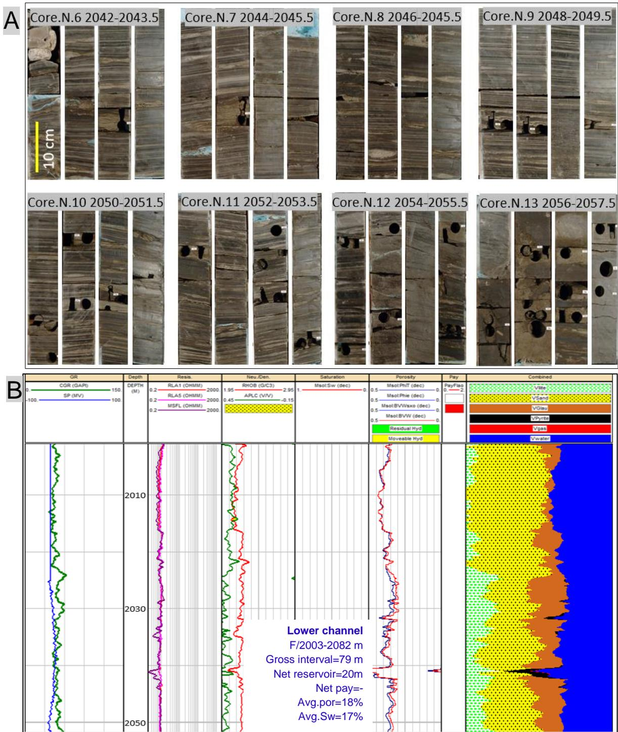
**Fig. 3.A:** Core photograph show the lower channel comprises of mainly well laminated silty mudstones with rare thin sandstones which interpreted as that outer slope deep marine. **B:** Litho-Saturation Cross-plot of lower channel in North Idkue – 4 well (interval 2000 - 2053 m)
