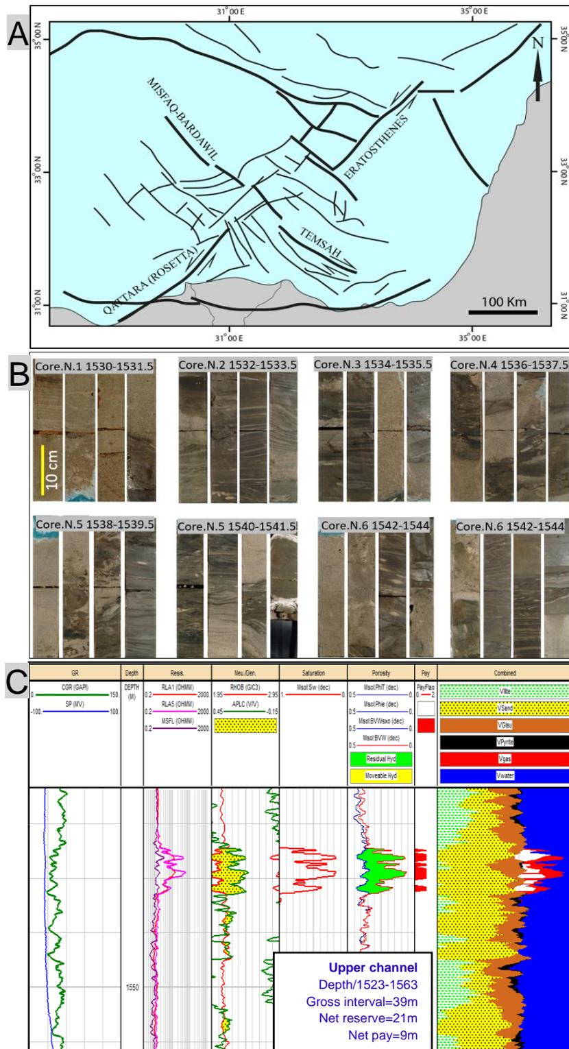
**Fig.2.A:** East Mediterranean structural domain with its main fault trends modified after Abd El Aasxl et. al.,(2000). **B:** Core photograph show the characteristics of lithology and reservoir rock properties of the upper channel. **C:** Litho-Saturation Cross-plot of upper channel in North. Idku – 4 well (interval 1479-1600)
