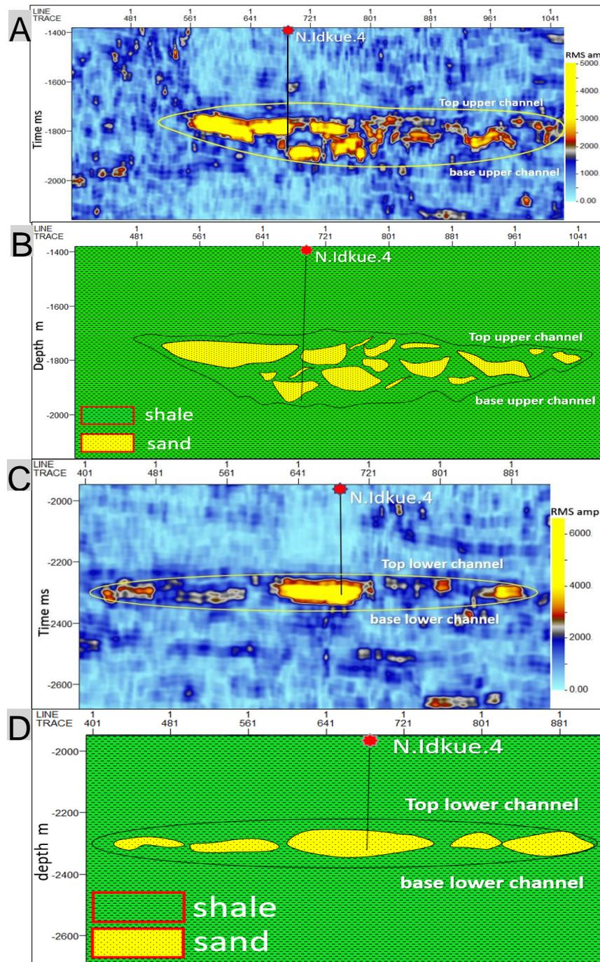
**Fig. 4.A:** Root-mean-square (RMS) amplitude cross section showing the upper channel interpreted as high amplitude value. **B:** Geoseismic section Crossline section showing the upper channel sands correspond with high amplitude value. **C:** Root-mean-square (RMS) amplitude cross section showing the lower channel interpreted as high amplitude value. **D:** Geoseismic section Crossline section showing the lower channel sands correspond with high amplitude value
