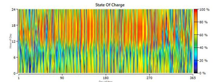
**Fig. 9:** The State of Charge (SOC) curve for the LI battery bank.
