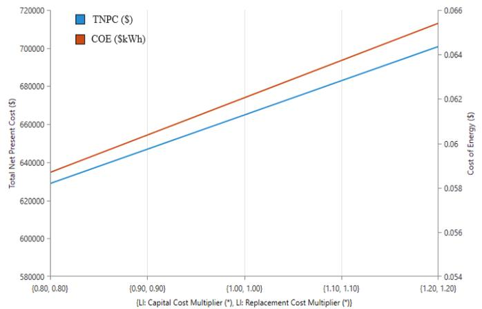
**Fig. 12:** Sensitivity analysis for Li-Ion Battery Bank cost variations on TNPC and COE of the proposed system.
