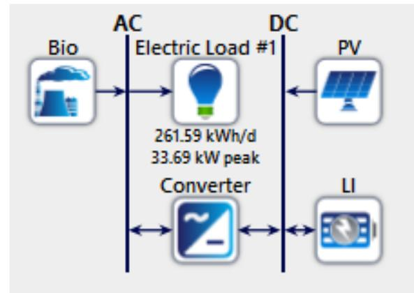
**Fig. 7:** The schematic diagram of the proposed system.
