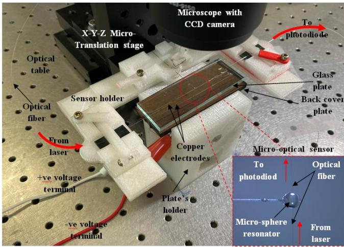
Fig. 3. A photograph of the experimental setup used to measure the electric field above a glass surface due to an applied voltage.
