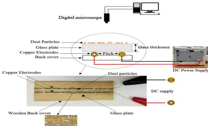
Fig. 6. A Schematic diagram of the experimental setup used for studying the removal of dust from the glass surface of PV panels by electrostatic forces.
