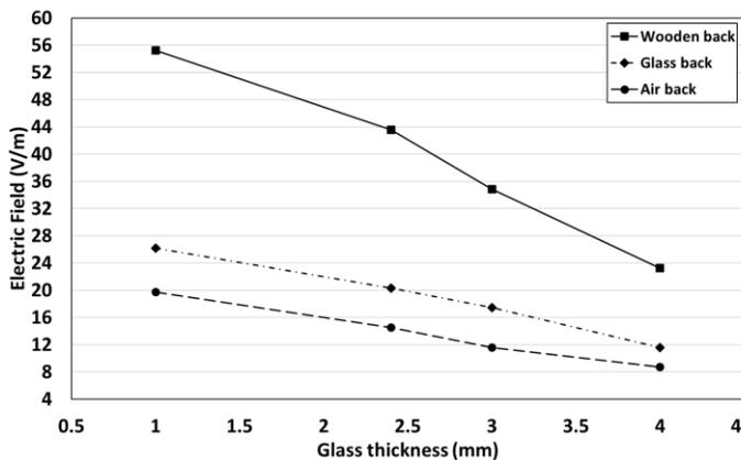
Fig. 4. The electric field above a glass surface as a function of the glass thickness and the back cover material; wood, glass and no cover, i.e. air.
