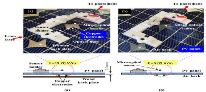
Fig. 5. The electric field above the glass surface of the PV panel as a function of the back cover material, i.e. (a) wood and (b) no cover, i.e. air.
