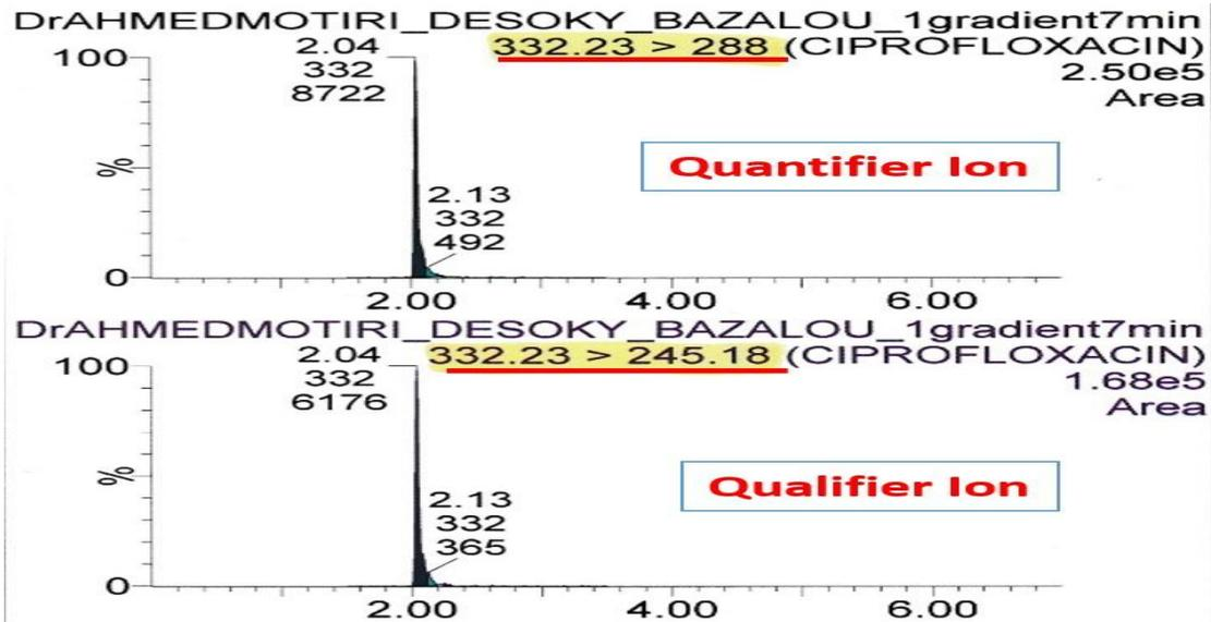
Fig. (2): Representative chromatogram showing quantifier and qualifier ions of ciprofloxacin as generated by the Quanpedia software and confirmed by the experimental work.
