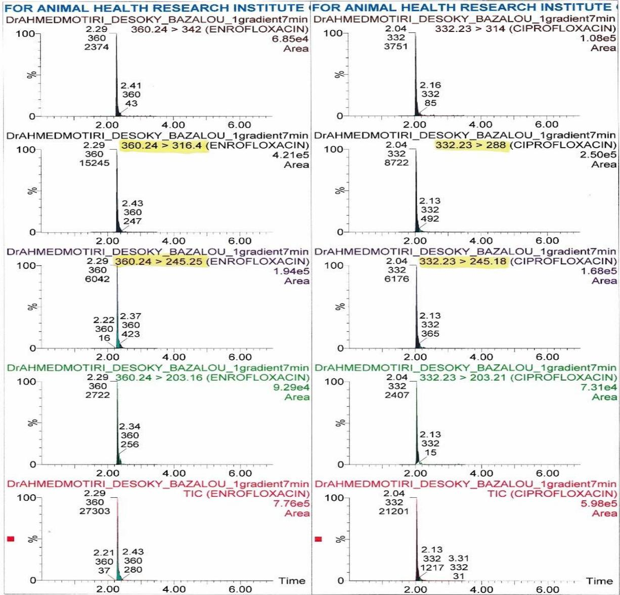
**Fig. (1):** Representative chromatogram showing total ion chromatograph (TIC) and daughter ions related to enrofloxacin and ciprofloxacin as generated by the Quanpedia software and confirmed by the experimental work.
