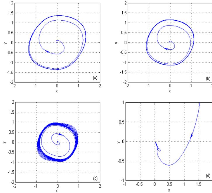
FIGURE 6. (a) Semi stable limit cycle in Lienard system with derivative order and initial value  $(x_0, y_0) = (0.001, 0.002)$ . (b) and (c) Semi stable limit cycle in Lienard system with order  $\alpha = 0.97$ , initial value  $(x_0, y_0) = (0.001, 0.002)$ , order  $\alpha = 0.9$  and initial value  $(x_0, y_0) = (0.001, 0.002)$ , respectively. (d) Limit cycle no longer exists in Lienard system with  $\alpha = 0.7$  and initial value  $(x_0, y_0) = (1, 2)$ .
