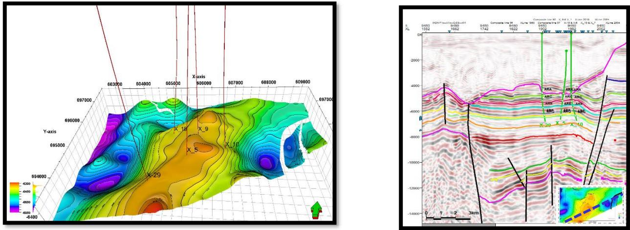
Fig. 4: AR "G" reservoir demonstrates the asymmetrical double plunging anticline that formed the WON X field and the interpreted seismic line
