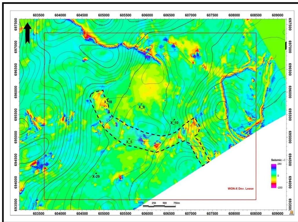
Fig. 6: instantaneous phase attribute map on top ARG+50 window illustrates the lateral variation in the reservoir that caused by structural or stratigraphic elements.
