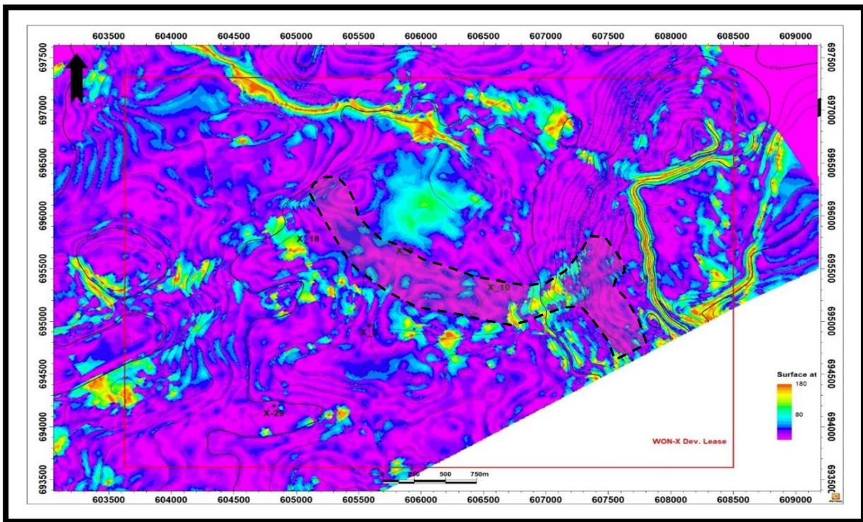
Fig. 5: RMS surface slice extracted on the top ARG reservoir, illustrating the variation in the amplitude resulted from the change in reservoir properties, as indicated by the black arrows.
