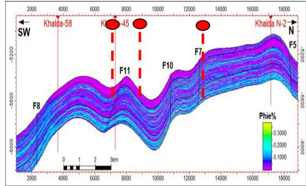
**Fig. 22:** N-SW cross-section illustrating effective porosity distribution in the main reservoirs in the study area with new prospect locations.
