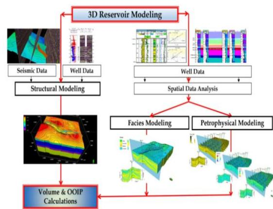
Fig. 4: Simplified workflow for 3D static reservoir modeling of Bahariya reservoirs in Khalda Oil Field, Western Desert, Egypt.
