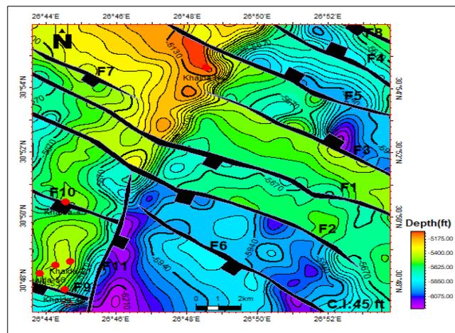
Fig. 5: Depth structure contour map on top of Upper Bahariya Reservoir.
