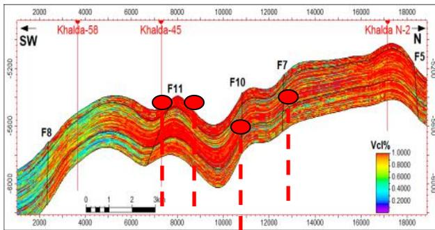
**Fig. 21:** N-SW cross-section illustrating clay volume distribution in the main reservoirs in the study area with new prospect locations.
