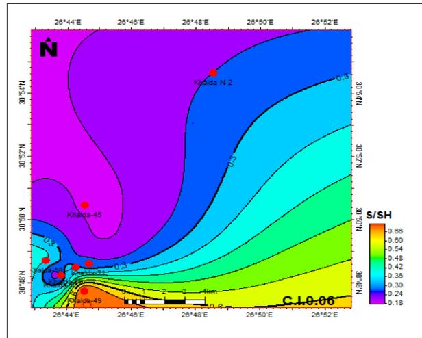
Fig.9: Sand/shale ratio map of Upper Bahariya Formation.
