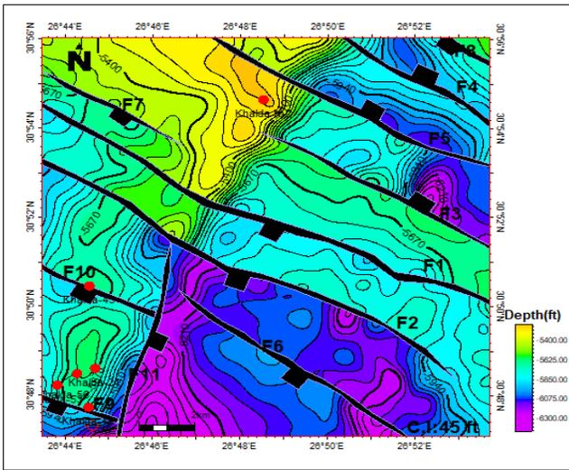
Fig. 6: Depth structure contour map on top of Lower Bahariya Reservoir.
