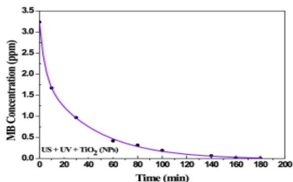
**Fig. 8:** Degradation activity vs. irradiation time during sonophotocatalysis process
