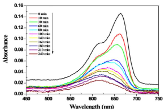
**Fig. 5:** UV-vis absorption spectra of MB solution catalyzed by TiO<sub>2</sub> NPs during the photocatalysis process.
