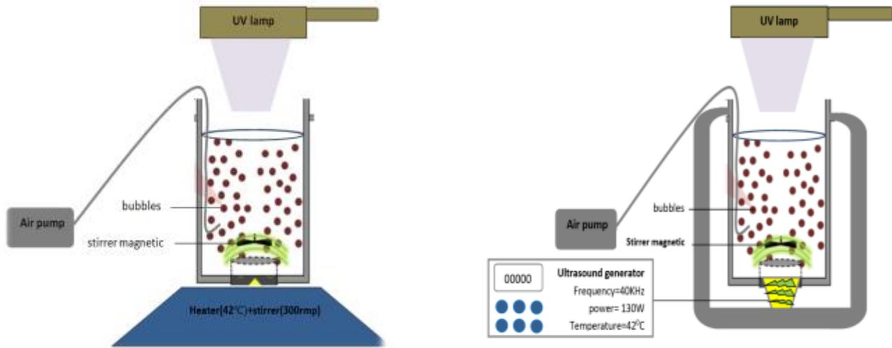
**Fig. 1:** Experimental set-up of (a) photocatalytic and (b) sonophotocatalytic reactors
