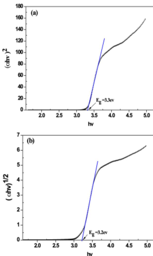
Fig. 4: Calculation of indirect band gap energy of TiO<sub>2</sub> NPs
