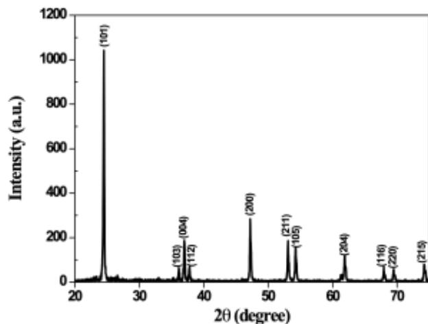
**Fig. 2:** XRD pattern of TiO<sub>2</sub> NPs
