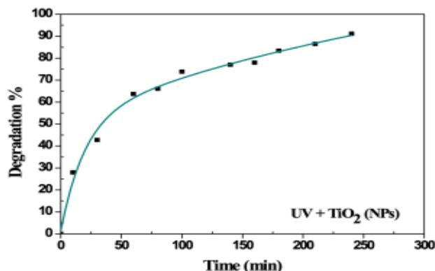
**Fig. 6** Degradation activity vs. irradiation time during the photocatalysis process.
