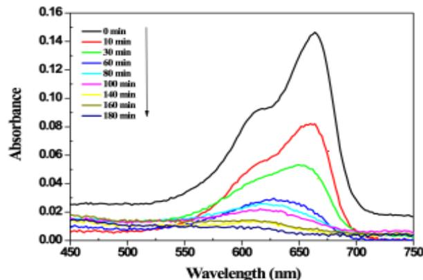
**Fig. 7:** UV-Vis absorption spectra of MB solution catalyzed by TiO<sub>2</sub> NPs during the sonophotocatalytic process.
