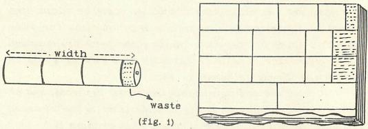
The company receives orders to cut, some of these reels or slices, to a set of sub reels of various width, suitable for the manufacturing necessities or the customer's demands. A number of cutting machines are at the disposal of the company, and their knives can be set for any combination of widths in which the total combined does not exceedthe overall roll width.
