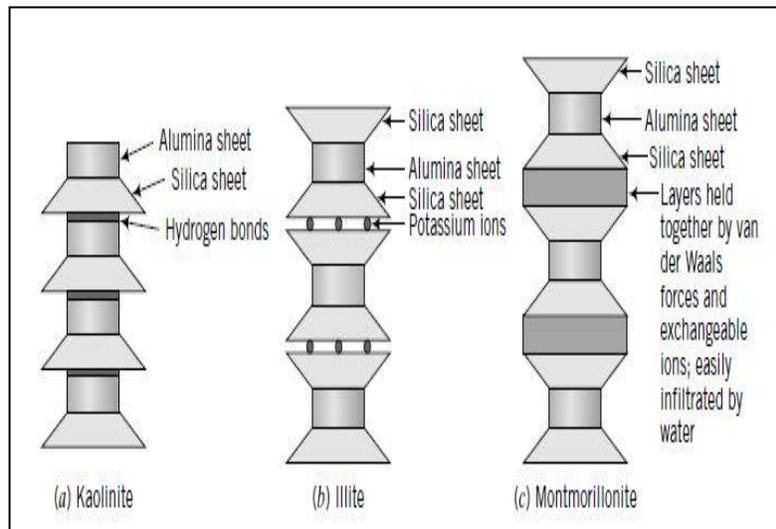
Figure1. Structure of Kaolinite, Illite, and Montmorillonite [11]
