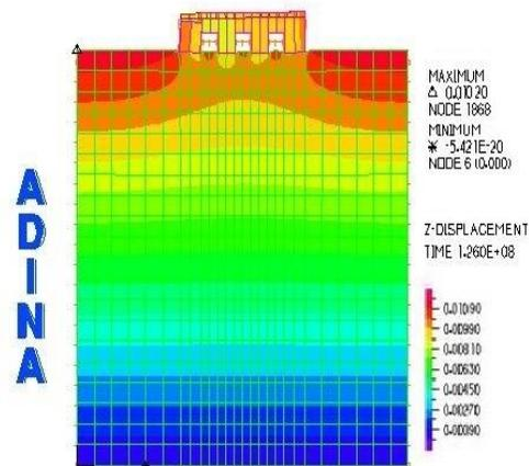
Figure 13. Numerical results for swelling soil and ribbed Geofoam with thickness=2 cm
