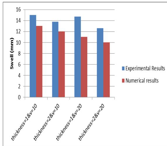
**Figure 15.** Comparison between Experimental and Numerical Results for Ribbed Geofoam
