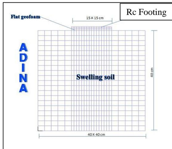
Figure4. Modeling of the steel plate footing with flat geofoam over the swelling soil
