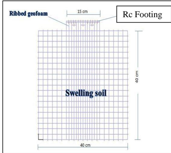
Figure5. Modeling of the steel plate footing with ribbed geofoam over the swelling soil
