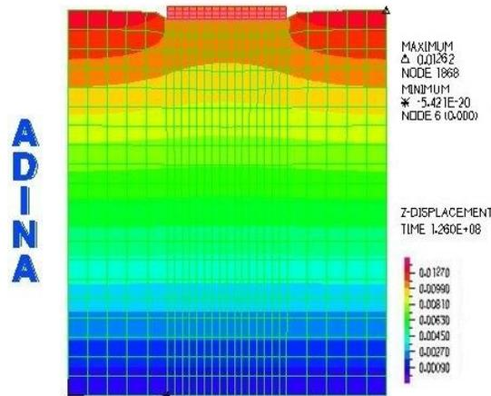
**Figure 10.** Numerical results for swelling soil and flat Geofoam with thickness=1cm
