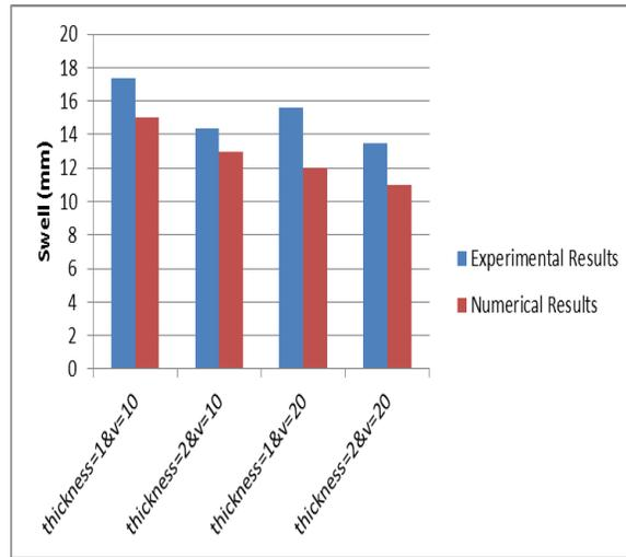
**Figure 14.** Comparison between Experimental and Numerical Results for Flat Geofoam
