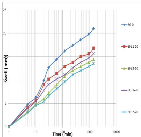
Figure 7. Soil heaves under different flat Geofoam
