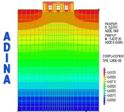
Figure 12. Numerical results for swelling soil and ribbed Geofoam with thickness=1 cm
