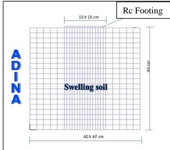
Figure3. Modelling of the footing over the swelling soil
