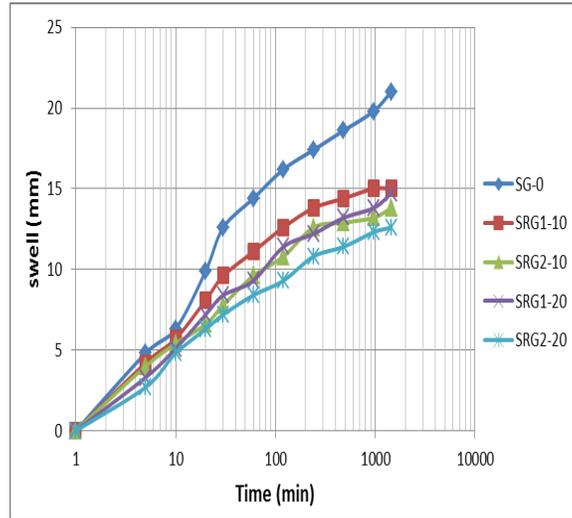
Figure 8. Soil heaves under different ribbed Geofoam
