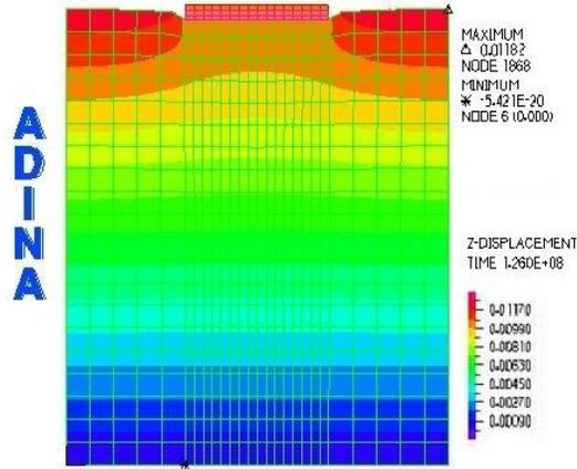
**Figure 11.** Numerical results for swelling soil and flat Geofoam with thickness=2 cm
