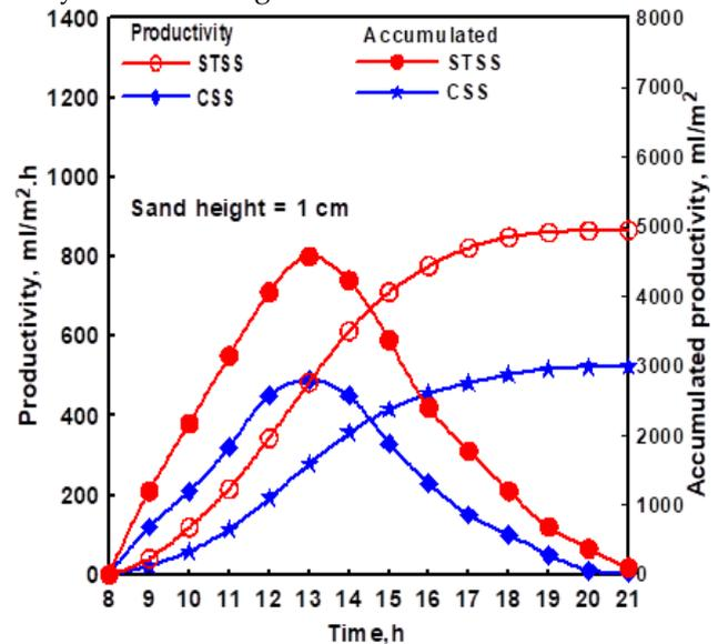
Fig. 5. The accumulated and hourly output production for tested SSs at sand height 1 cm
