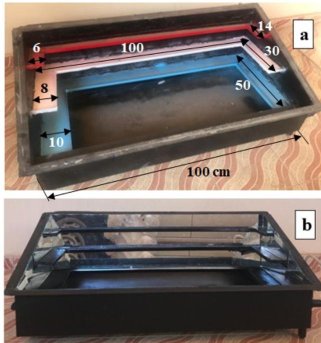
Fig. 3. TSS (a) without black paint, (b) with black paint with internal mirrors.
