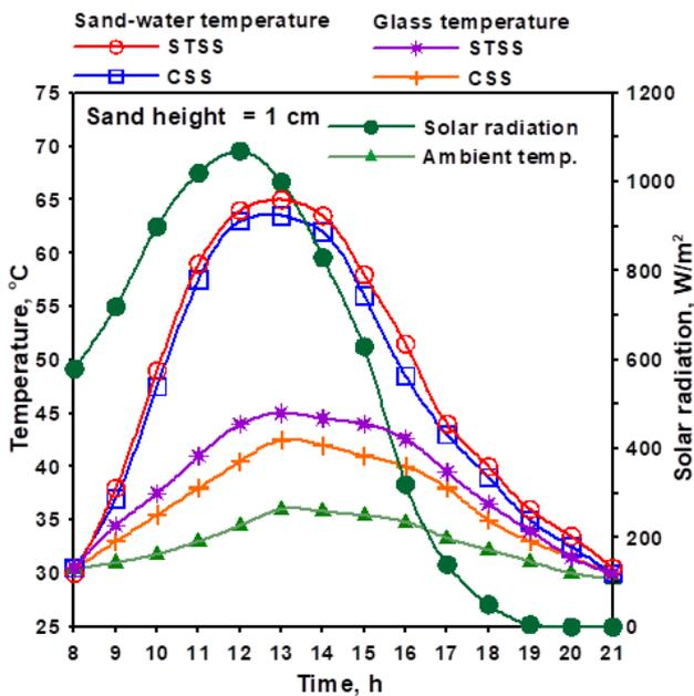
Fig. 4. Solar radiation and temperatures profiles for tested SSs at sand height 1 cm.
