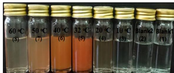
**Figure 10.** The synthesis of selenium nanoparticles is indicated by the various colors acquired from the selenium reduction assay at various temperatures. The numbers (1-2) represent the corresponding blank reactions, while the numbers (3-8) represent *Streptomyces sp* culture reactions with 2 mM Na<sub>2</sub>SeO<sub>3</sub> at pH 7, incubation at various temperatures as specified (10, 20, 32, 40, 50, and 60 °C) respectively.
