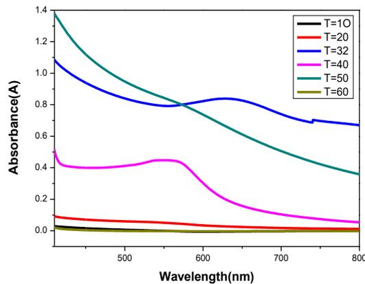
**Figure 11.** Selenium nanoparticle production may be seen in the UV-Vis absorption spectra of the surface Plasmon resonance recorded for the various temperatures as a change in the absorbance around 582 nm - 650 nm.
