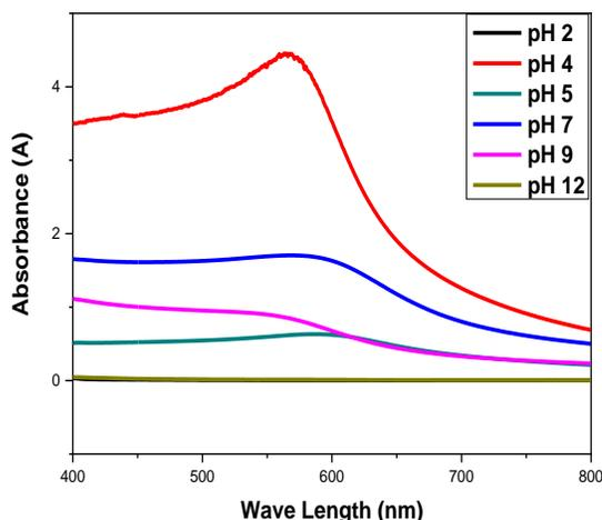
**Figure 9.** According to the surface Plasmon resonance, UV-Vis absorption spectra acquired for the various pH values, selenium nanoparticle formation is indicated by a change in the absorbance around 582 nm.
