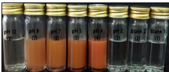
**Figure 8.** The synthesis of selenium nanoparticles is indicated by the various colors produced from the selenium reduction assay at various pH levels. The tubes with numbers (1-2) represent blank reactions, whereas those with even numbers (3-8) represent *Streptomyces sp* culture reactions with 2mM of Se<sub>2</sub>NaO<sub>3</sub> at pH 2, 4, 5, 7, 9, and 12 accordingly.
