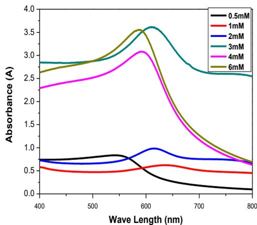
**Figure 7.** Spectra of UV-Vis absorption of selenium nanoparticles solution after the reaction of different concentrations of aqueous Na<sub>2</sub>SeO<sub>3</sub> solution at neutral pH with the bacteria *Streptomyces sp* culture for 5-7 days.
