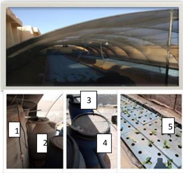
**Fig. 1:** A newly developed DWC, a prototype built in the Upper Egypt Center of Development owned by the ASRT in Sohag Governorate, Egypt (1- Fish tank, 2- Mechanical filter, 3- Net filter, 4- Biofilter, 5- Hydroponic part).
