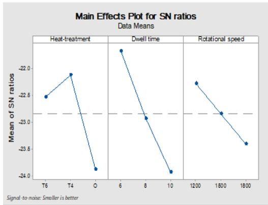
Fig 8 The main effect plot for S/N ratio for average grain size.
