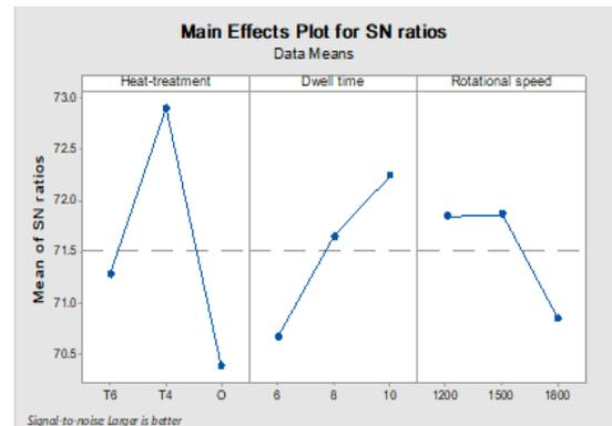
Fig 7 The main effect plot for S/N ratio for shear load.
