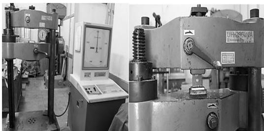
Fig 3 Computerized tensile testing machine.
