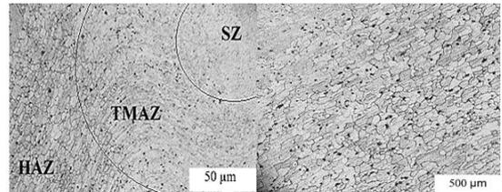
Fig 4 Macrostructure of HAZ, Fig 5 Microstructure of SZ at TMAZ and SZ at 1200 rpm and 6 sec.1500 rpm and 10 sec.
