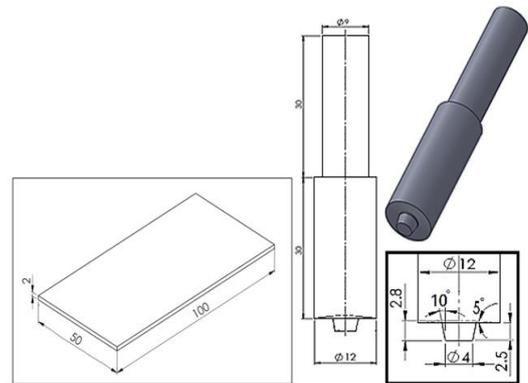
Fig 1 Specimen dimensions. Fig 2 Dimensions of rotating tool.
