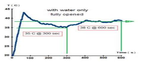
This figure reflects the poor effect of using water only on the fire extinguishing, during 600 sec the sprayed water couldn't extinguish the fire
