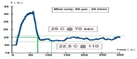
Figure 9. "Average Temperature of using water mist only (Q= 500 kW/m², q mist= 20 l/min, Di= 50 μm)"
