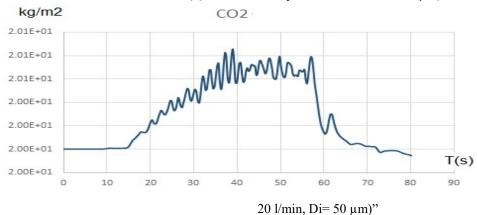
Water mist nozzles activations affect extremely positively on both of carbon dioxide concentration and the heat flux.
