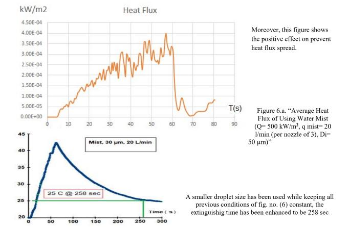
Figure 7. "Average Temperature of Using Water Mist (Q=  $500 \text{ kW/m}^2$ , q= 20 l/min (per nozzle of three), Di=  $30 \mu\text{m}$ )"
