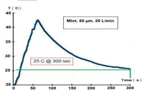
In this fig. no. (6), once applying the water mist fire suppressing system to the same model of previous fig. no. (5), a pronounced effect has been occurred, and finally the fire is extinguished @ 300 sec.
