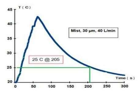
After double the quantity of flow rate amount to be (40 l/m), maintaining all conditions the same as previous fig. no. (7), an enhancement in time of fire extingiuishing has been occurred by more than 50 sec to be reached 205 sec
