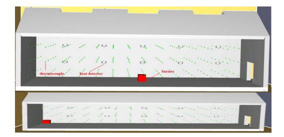
Figure 3. "Schematic 3D view of hanger model (FDS)"
