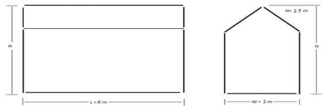
Figure 2. "Elevation and Side View of hanger model"
