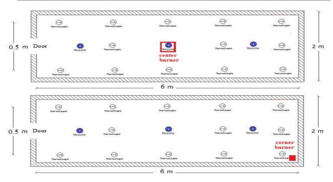
Figure 1. "Plan of hanger model"
