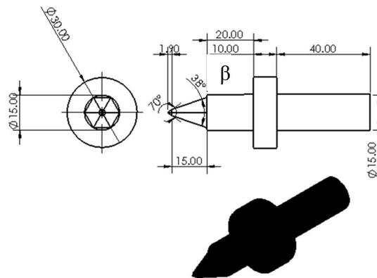
Figure 1. (a) The dimensions of the tool with hexagonal shape and conical angles ( $\beta$ ). The conical angle has values of  $38^\circ$ ,  $42^\circ$  and  $58^\circ$ .
