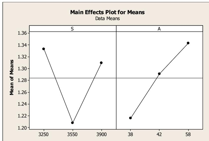
Figure 6. Main effects plot for means of the bushing wall-thickness.
