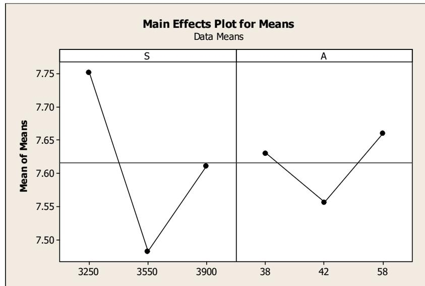
Figure 5. Main effects plot for means of the bushing height.
