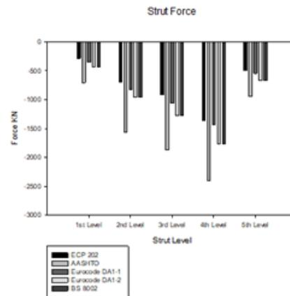
Fig. [6] Strut forces for case 1 in medium dense sand
