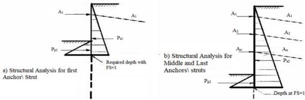
Fig. [1] Analysis method of a multi-level strutted or anchored excavation (reproduced from ECP 202).
