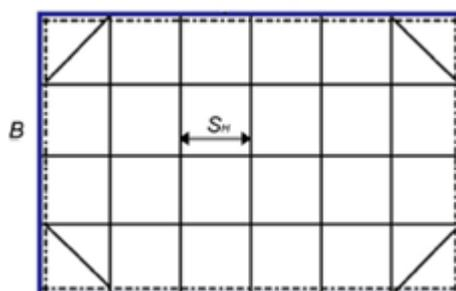
Fig. [3] (3): horizontal spacing between struts
