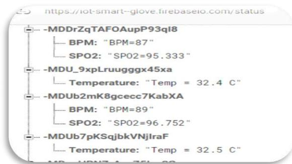
FIG 5:Practical sensors readings in web server “Firebase”
