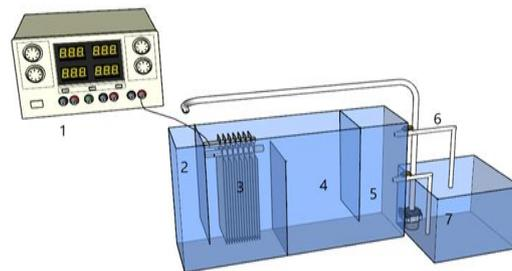
Fig (2): A schematic Diagram of the E.C (1. DC Power source. 2. Water inlet. 3. Al Electrodes. 4. Flotation unit. 5. Settling unit. 6. Water outlet. 7. Final storage and circulation pump)
