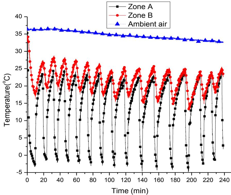
**Figure 5.** The variation in the temperatures of zone A, zone B and ambient air with time at 30% relative humidity.
