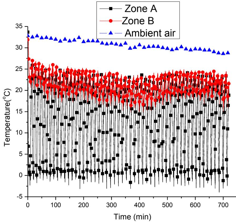
**Figure 8.** The variation in temperatures with time for zone A, zone B and ambient air at 81-100% relative humidity.
