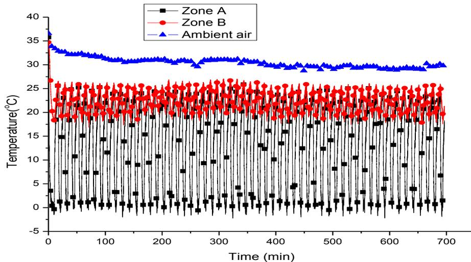
**Figure 14.** The variation in temperatures with time for zone A, zone B and ambient air temperature at 65-97% relative humidity.
