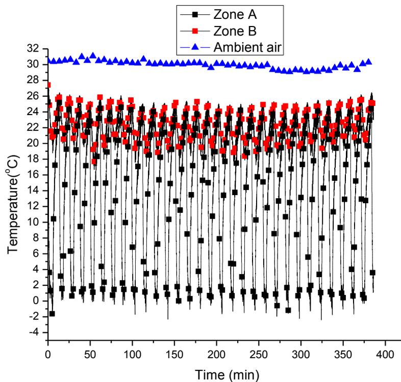
**Figure 11.** The variation in the temperatures with time for zone A, zone B and ambient air at 81-86% relative humidity.
