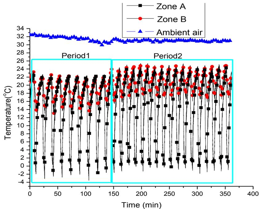
**Figure 10.** The variation in the temperatures with time for zone A, zone B and ambient air at 79-100% relative humidity.
