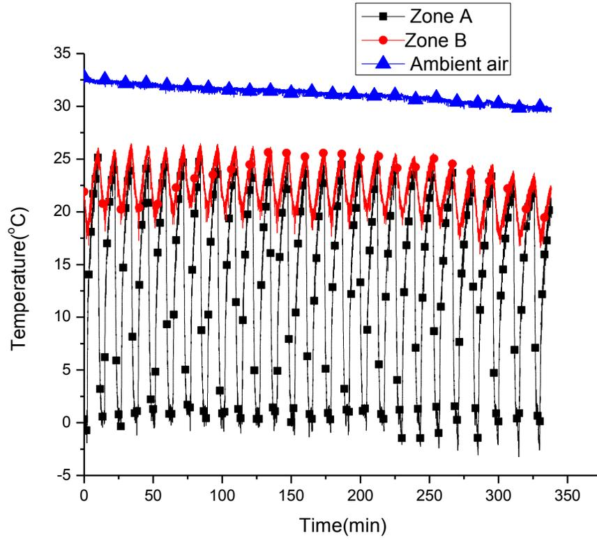
**Figure 6 .** The variation in temperatures with time for zone A, zone B and ambient air at 66-72% relative humidity.
