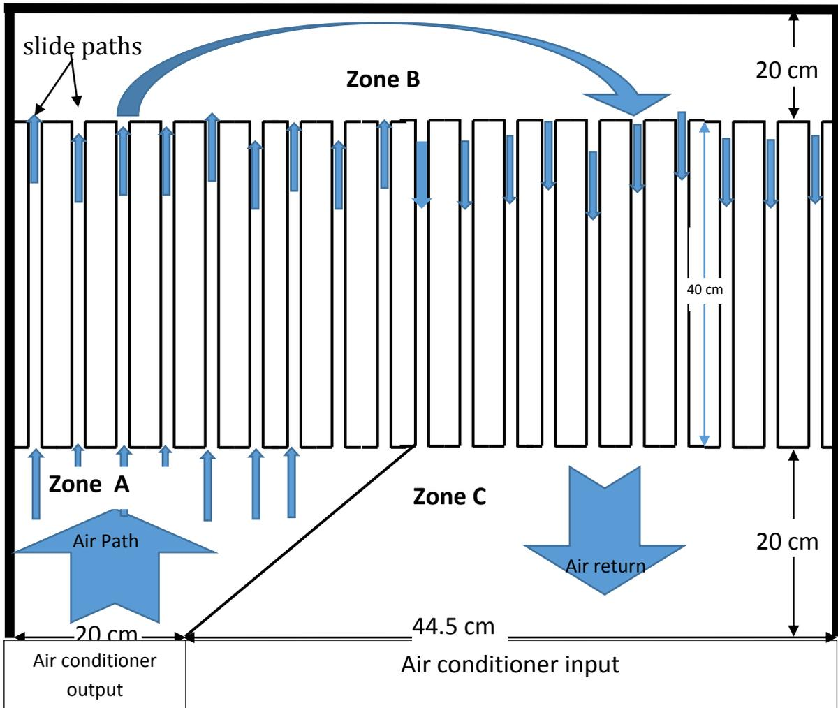
**Figure 1.** Schematic diagram of the attachment.
