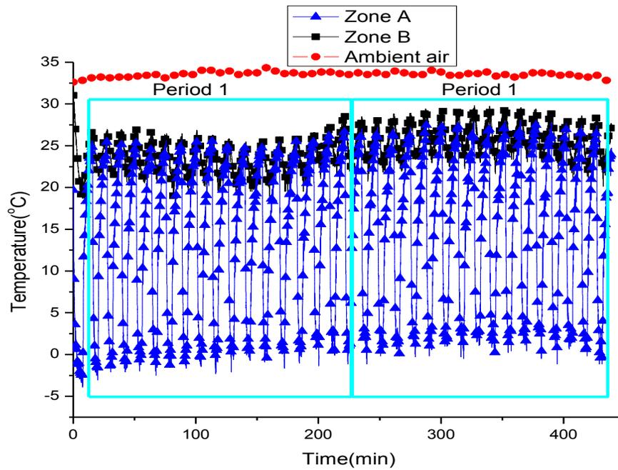
**Figure 12.** The variation in temperatures with time for zone A, zone B and ambient air at 72-92-82% relative humidity.
